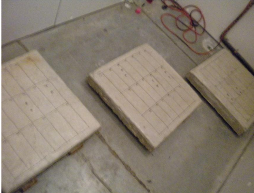
Figure 3-12: Concrete slabs prepared for experimentation on concrete material variables.
