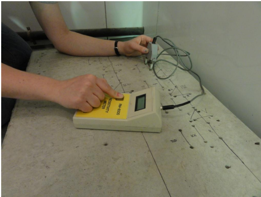
Figure 3-10: Two-prong resistivity testing.
