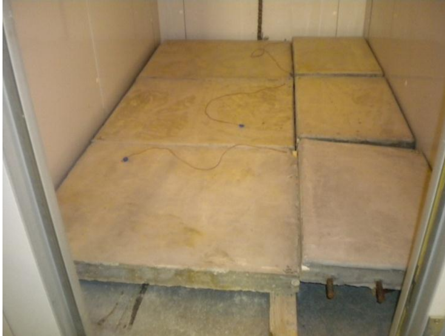
Figure 3-7: Concrete slabs prepared for experimentation on operator-controlled variables.
