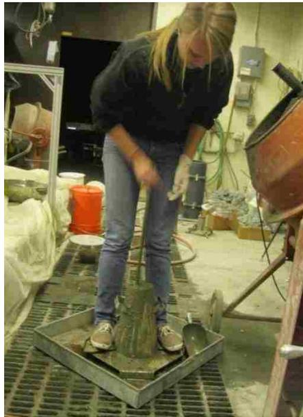
**Figure 6. Slump Cone with Grout Type 6**
