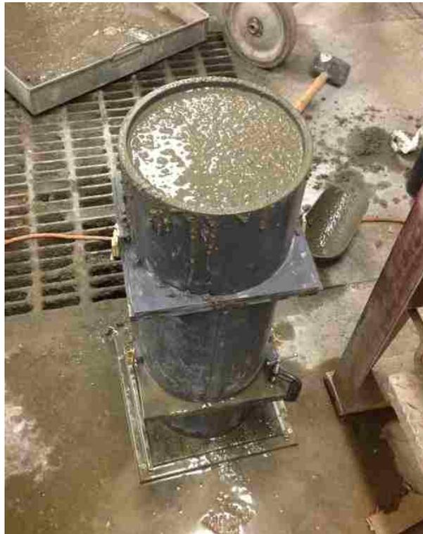
**Figure 10. Segregation Column with Grout Type 5**
