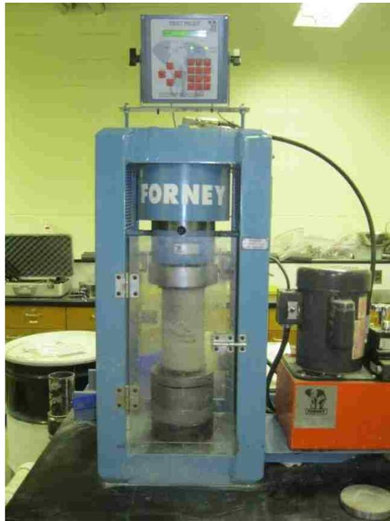
**Figure 13. Grout Specimen Compressive Testing**
