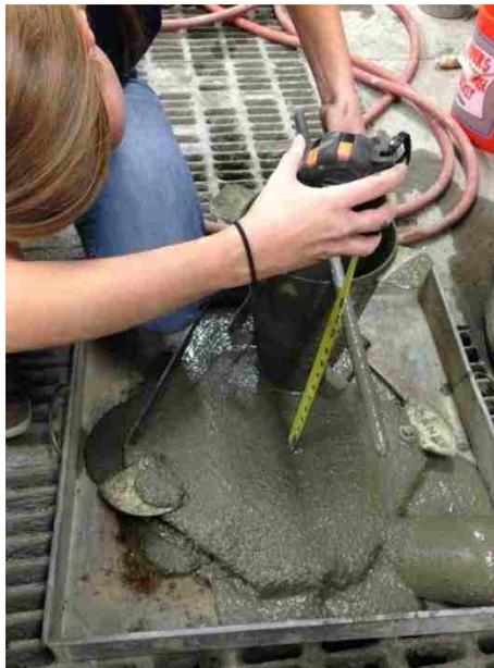
**Figure 7. Grout Slump Measurement with Grout Type 3**
