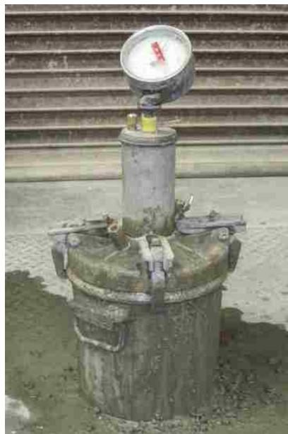
**Figure 9. Air Content by the Pressure Method**
