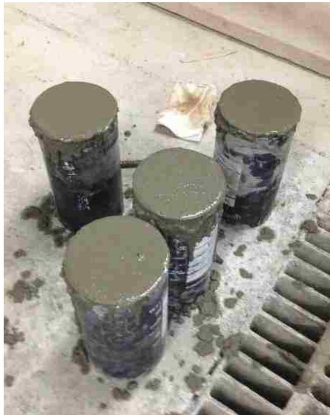
**Figure 11. Grout Type 1 Cylinder Specimens**
