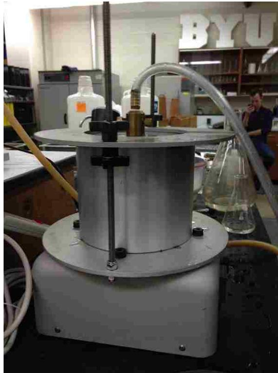
**Figure 4. Coarse Aggregate Testing with Vacuum Pump**
