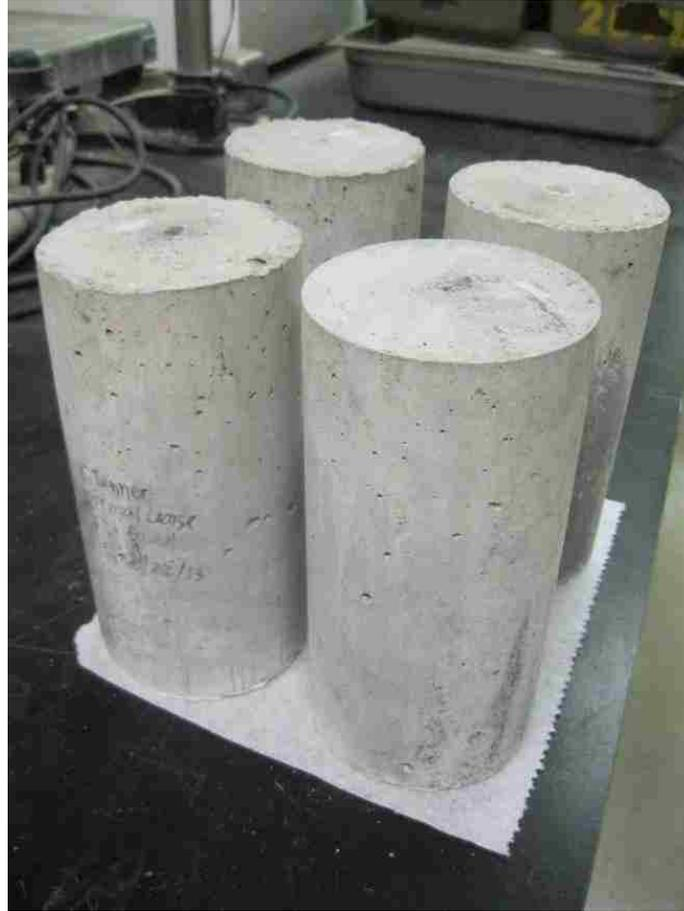
**Figure 12. Grout Type 5 Cylinder Specimens**
