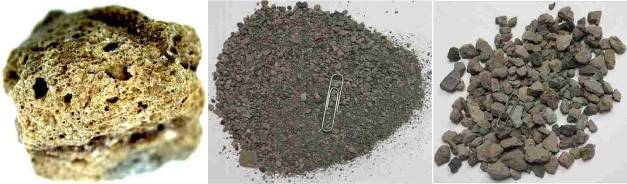
Figure 1. Expanded Shale Close-up (Left), Crushed Fines (Middle), Coarse (Right)
