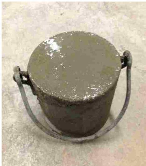
**Figure 8. Unit Weight Bucket with Grout.**
