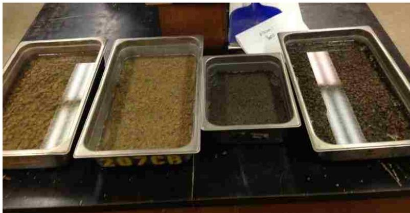
**Figure 2. Aggregate Soaking**
