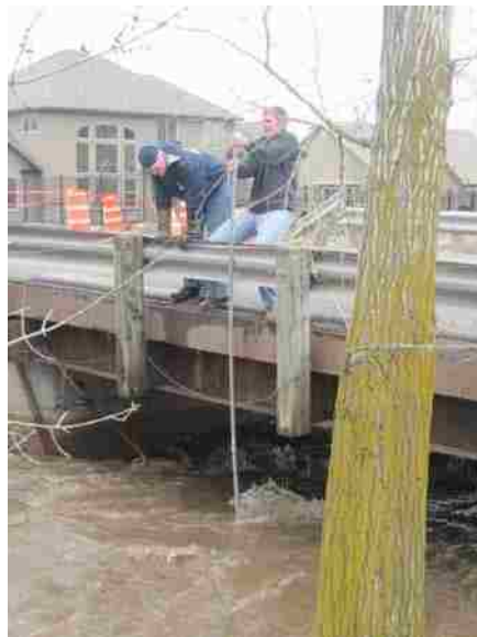
Figure A.5: Inappropriate sampling caused excessive strain on Stanley Sampler.
