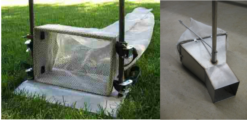
Figure A.2: Net trap sampler (left) and Helley-Smith sampler (right)
