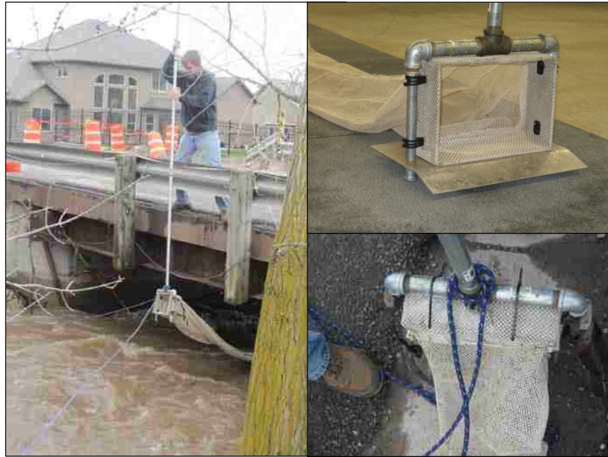
Figure A.4: Pole-mounted Net Trap Sampler, or Stanley Sampler: in the lab (bottom right), in the field (top right), and suspended above Hobble Creek (left).
