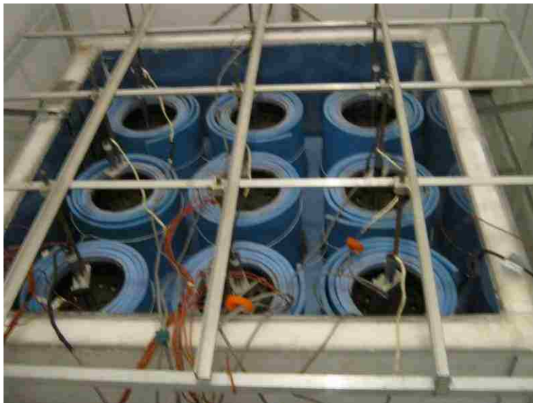
Figure 3-13: Frost heave test configuration.
