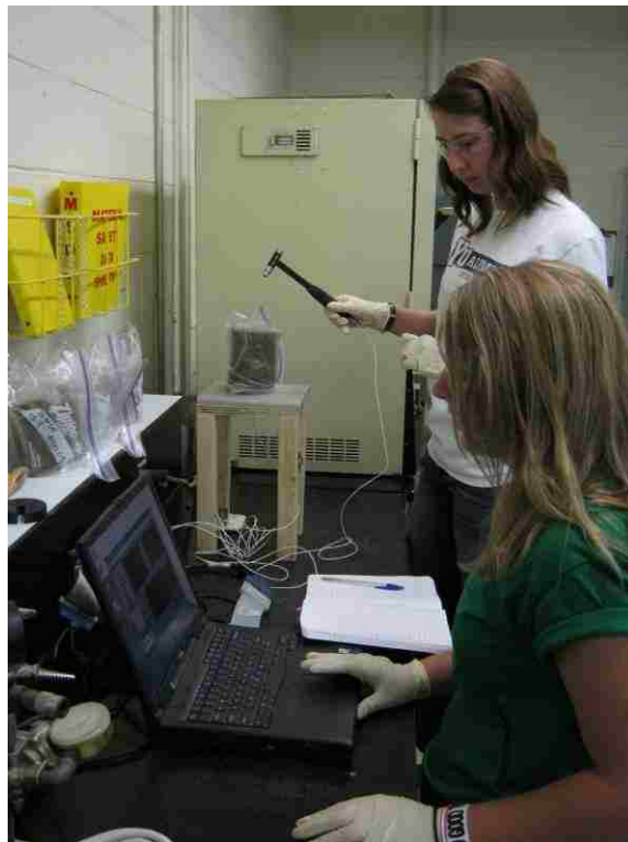
Figure 3-8: Modulus testing of a freeze-thaw specimen.
