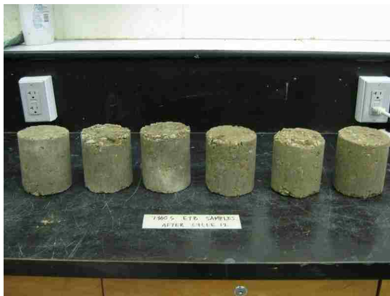
Figure 3-7: Freeze-thaw specimens from 7800 South.
