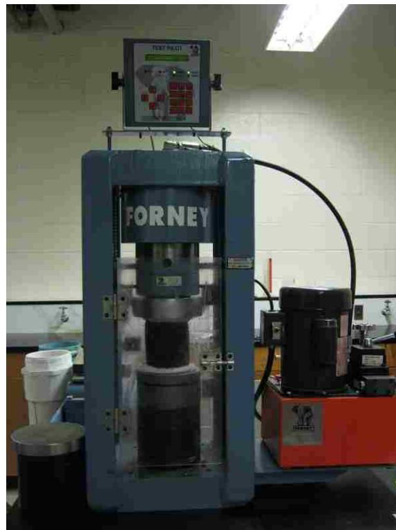
Figure 3-11: Unconfined compressive strength testing of a freeze-thaw specimen.
