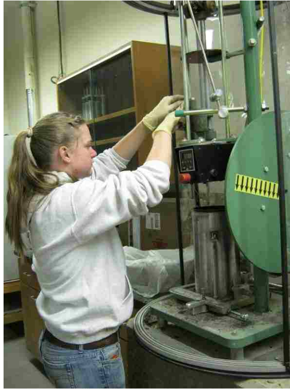
Figure 3-12: Compaction of a frost heave specimen.
