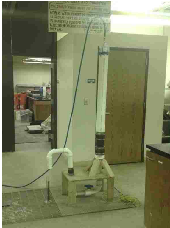
Figure 3-15. Permeability test configuration.
