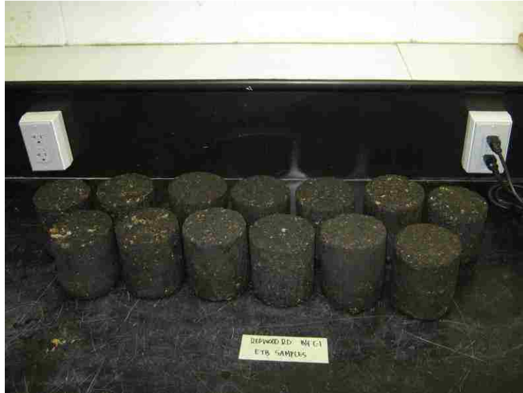
Figure 3-6: Freeze-thaw specimens from Redwood Road.
