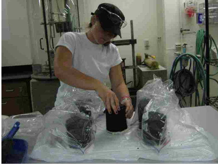
Figure 3-10: Capping of a freeze-thaw specimen.
