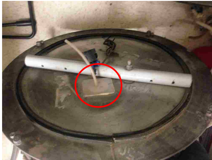
Figure 5: Chamber Lid with Added Plated Attached as Indicated by Red Circle
