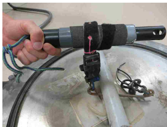
Figure 4: Mounting Mechanism with Probe Attached
