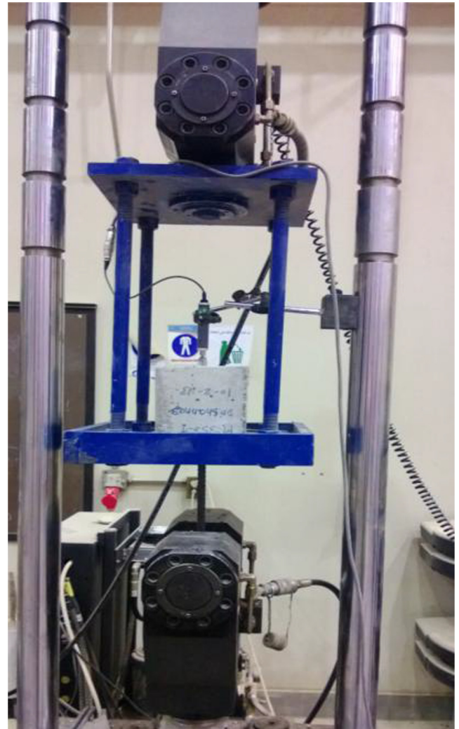
Fig. 3. INSTRON testing machine showing a tested specimen.
