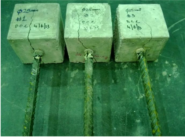
Fig. 5. Pull-out specimens after testing ( l_e = 150 mm).
