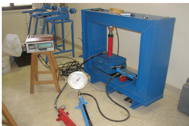
Figure 8 Manufactured large scale direct shear device.
