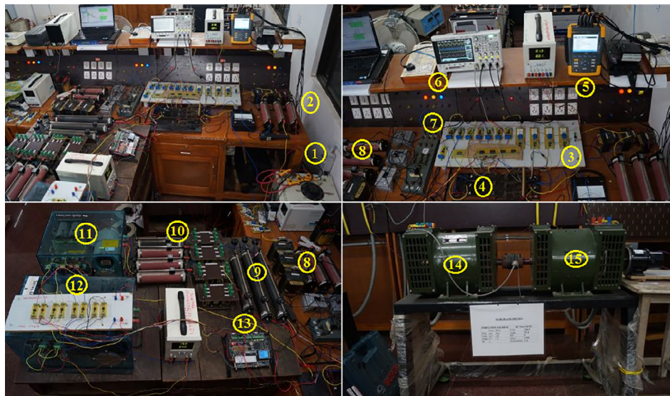
Fig. 7. Snap shot of the implemented FL-DSTATCOM in the HES laboratory. (1) 3-phase supply (2) Feeder (3) Signal conditioning and acquisition circuit (4) PCC (5) Fluke meter (6) DSO (7) Load switch (8) Static load (9) RC filter (10) RL filter (11) FL-DSTATCOM (12) Gate driver circuit (13) FPGA board (14) Dynamic load (SRIM) (15) DC machine.
