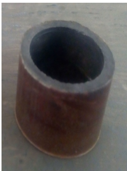
Plate 1 Banana stem (particulate) reinforced PVC composite pipe.
