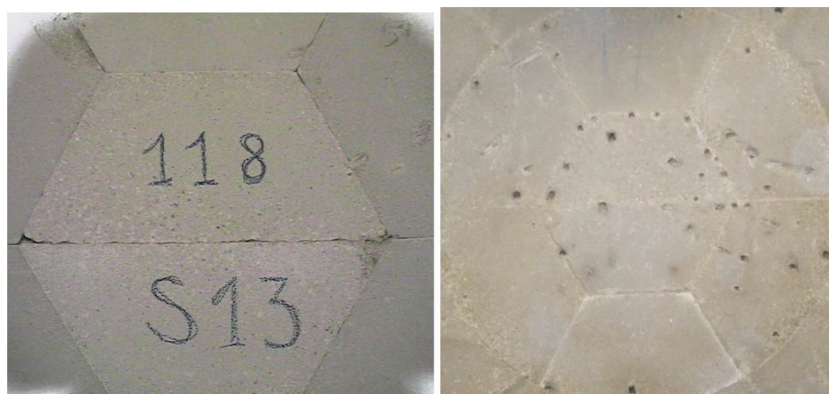
Fig. 9. Appearance of the core of the barrier in cold zones after 5 years (left, slice 118, section S13) and 18 years (right, slice 17, section S57–S58).
