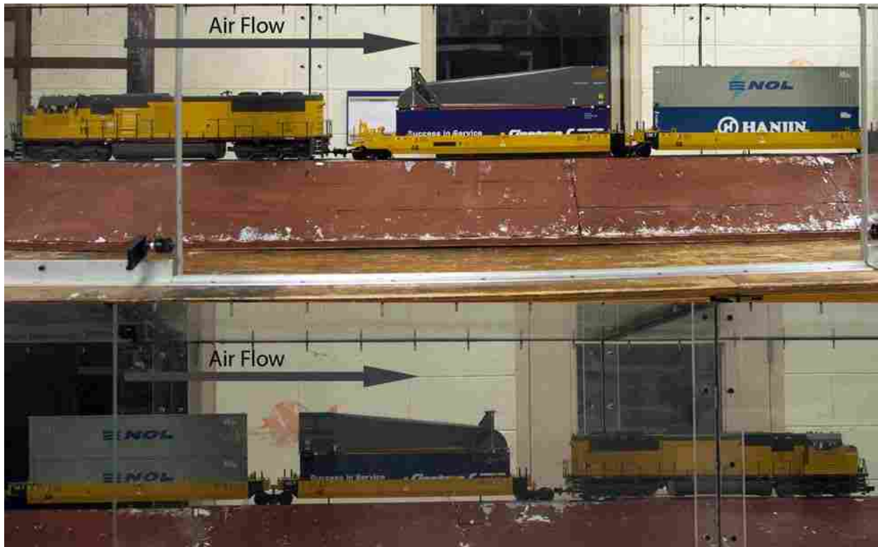
Figure 3.13: Image of the model that was tested at both the front(top panel) and the rear of the train(bottom panel).
