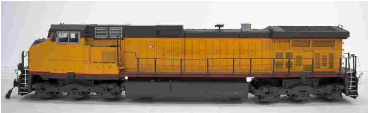
Figure 2.3: G-Scale locomotive train model. These models were purchased from a model train manufacturer and placed at the front of the wind tunnel test track. Drag on the locomotives was not measured in this study.
