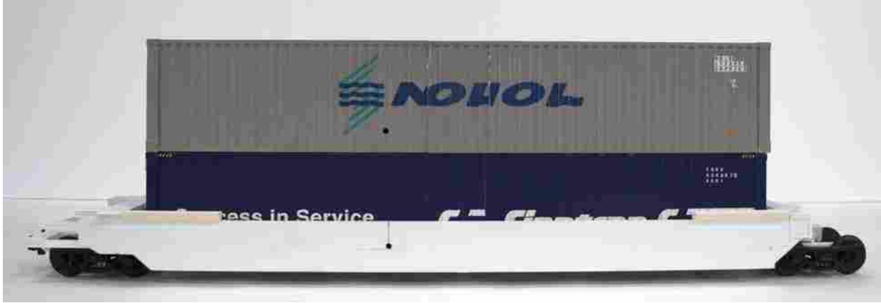
Figure 2.9: Image of a 53 ft. well car model loaded with double stacked 53 ft. containers. Actual container model length is approximately 55 cm.
