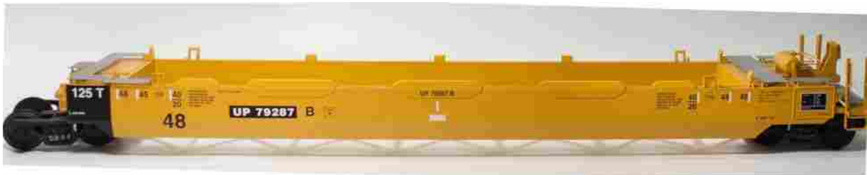
Figure 2.6: Image of 48 ft. well car model. Length refers to the recessed well and not the total rail car length.
