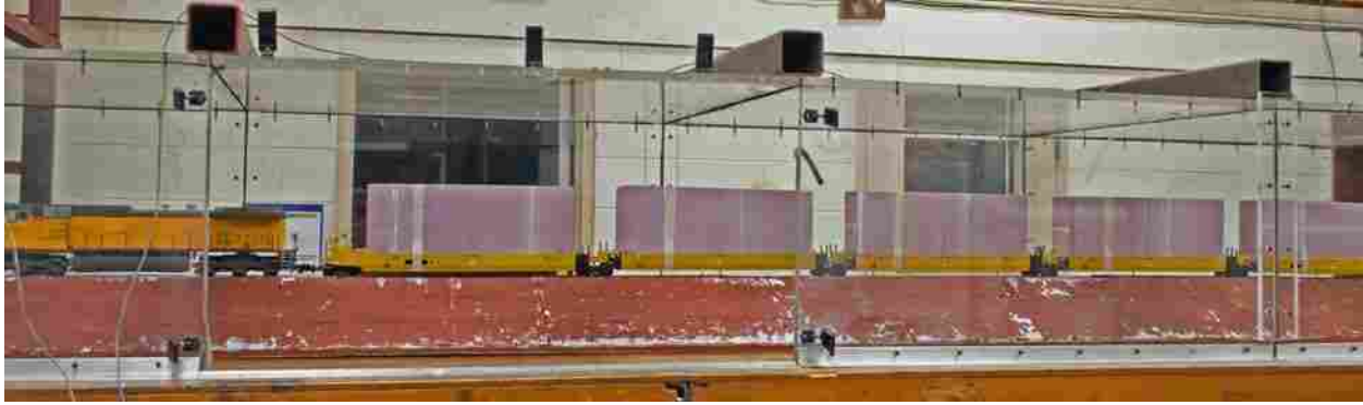
Figure 3.8: Foam containers constructed to study the effect of the container gap on the drag.
