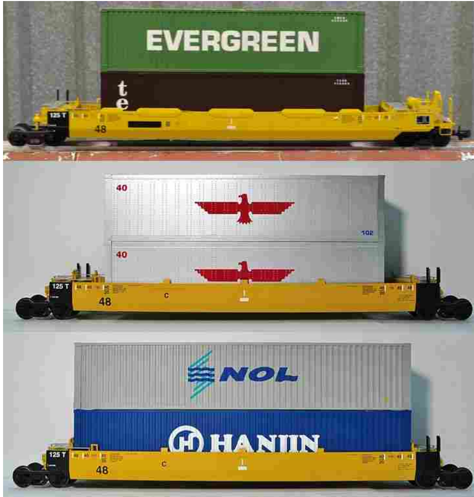
Figure 3.2: Images of container models utilized in the 48 foot well car models. Corrugated 40 foot containers are shown in the top panel; smooth 40 foot containers are shown in the middle panel; corrugated 48 foot containers are shown in the bottom panel.
