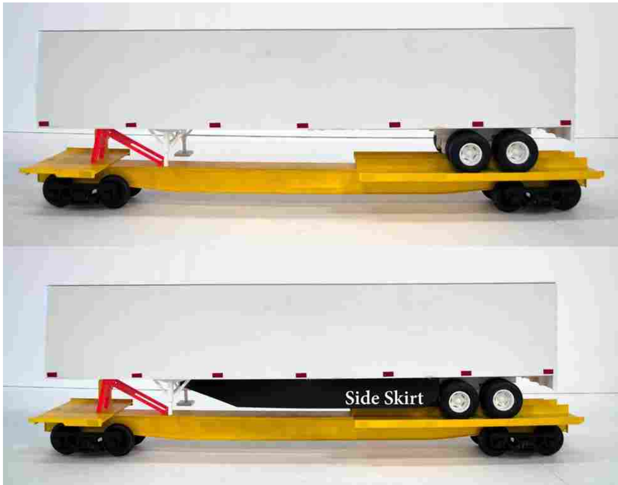
Figure 2.13: Side images of a semi-trailer on a 53' spine car model. The top panel shows a semi-trailer without a side skirt and the bottom panel shows a semi-trailer with a side skirt.
