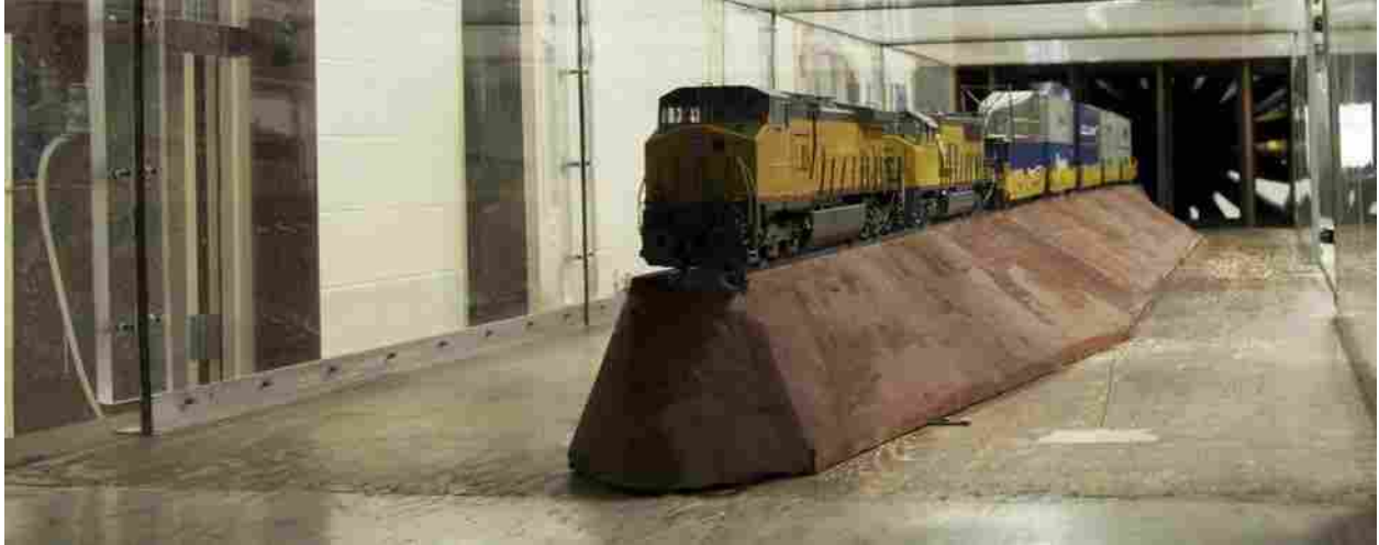
Figure 2.1: The test track and model system was constructed and secured to the wind floor. The track was used to simulate the flow past actual rail cars and each rail car was fastened to the test track. Force data was collected from individual intermodal rail cars with a system of load cells.
