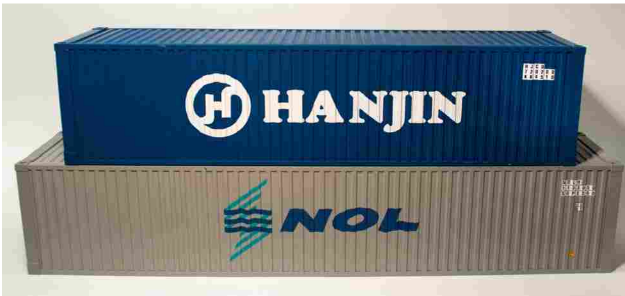
Figure 2.8: 40 ft. corrugated container model stacked on a 48 ft. container model. Actual model lengths are approximately 42 cm and 50 cm respectively.
