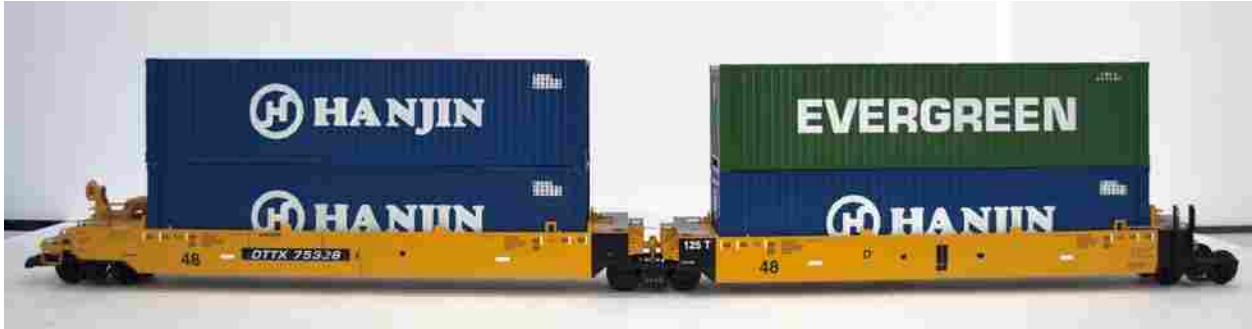
Figure 2.7: Image of two 40 ft. articulated well car models loaded with double stacked 40 ft. containers.
