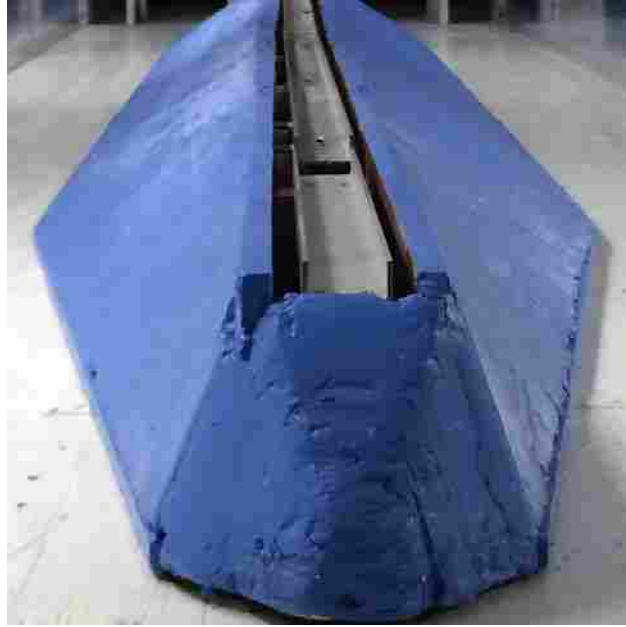
Figure 2.2: Sections of channel aluminum were used for the rail car track. These sections could be rearranged or replaced to accommodate different rail car lengths.
