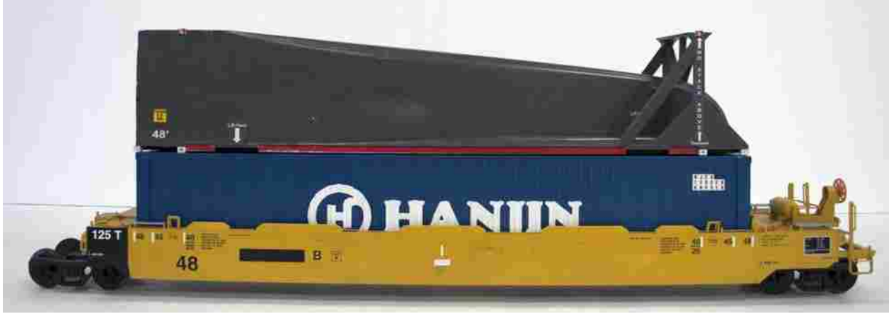
Figure 2.10: Image of the Union Pacific Arrowedge® model used to reduce the drag on the first and last container cars. The Arrowedge® is stacked on a 48 ft. container loaded in a 48 ft. well car.
