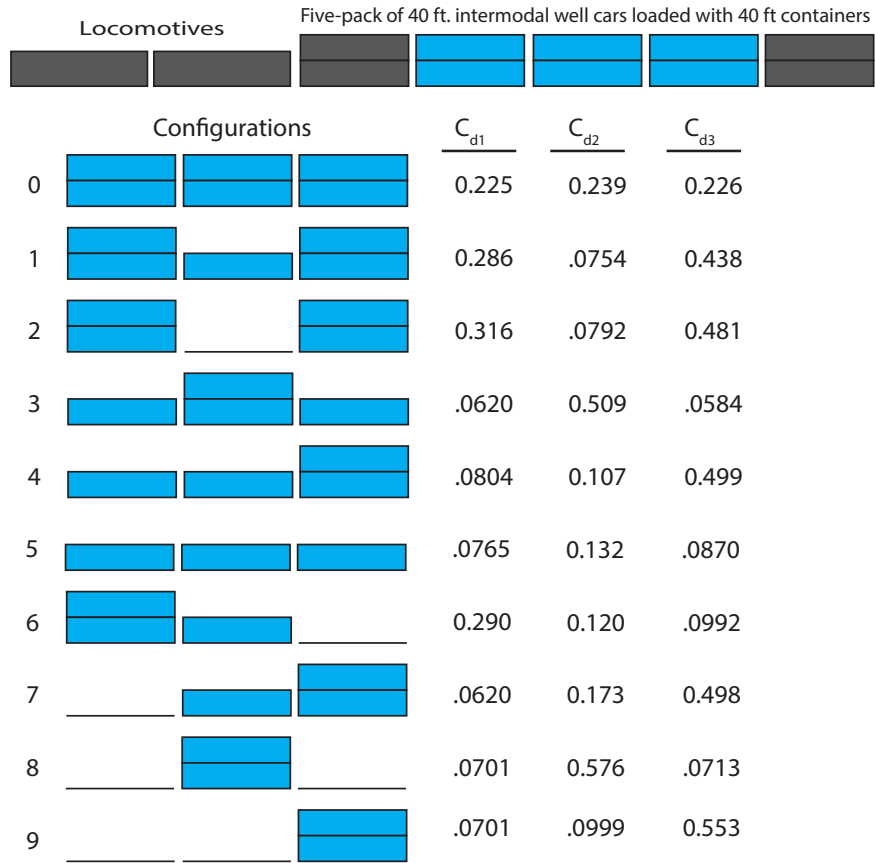
Figure 3.3: Average drag coefficients for partial load configurations with a set of five 40 foot well cars.
