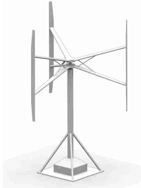
Figure 1.2: A computer model based on the 12 kW H-rotor VAWT found at Uppsala University in Sweden [3].
