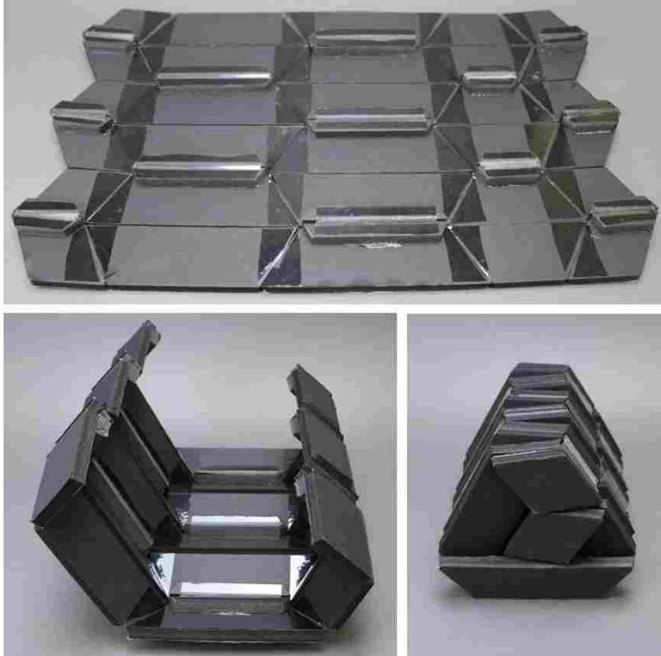
Figure 5.1: Origami-adapted mechanism shown flat, partially folded, and folded.
