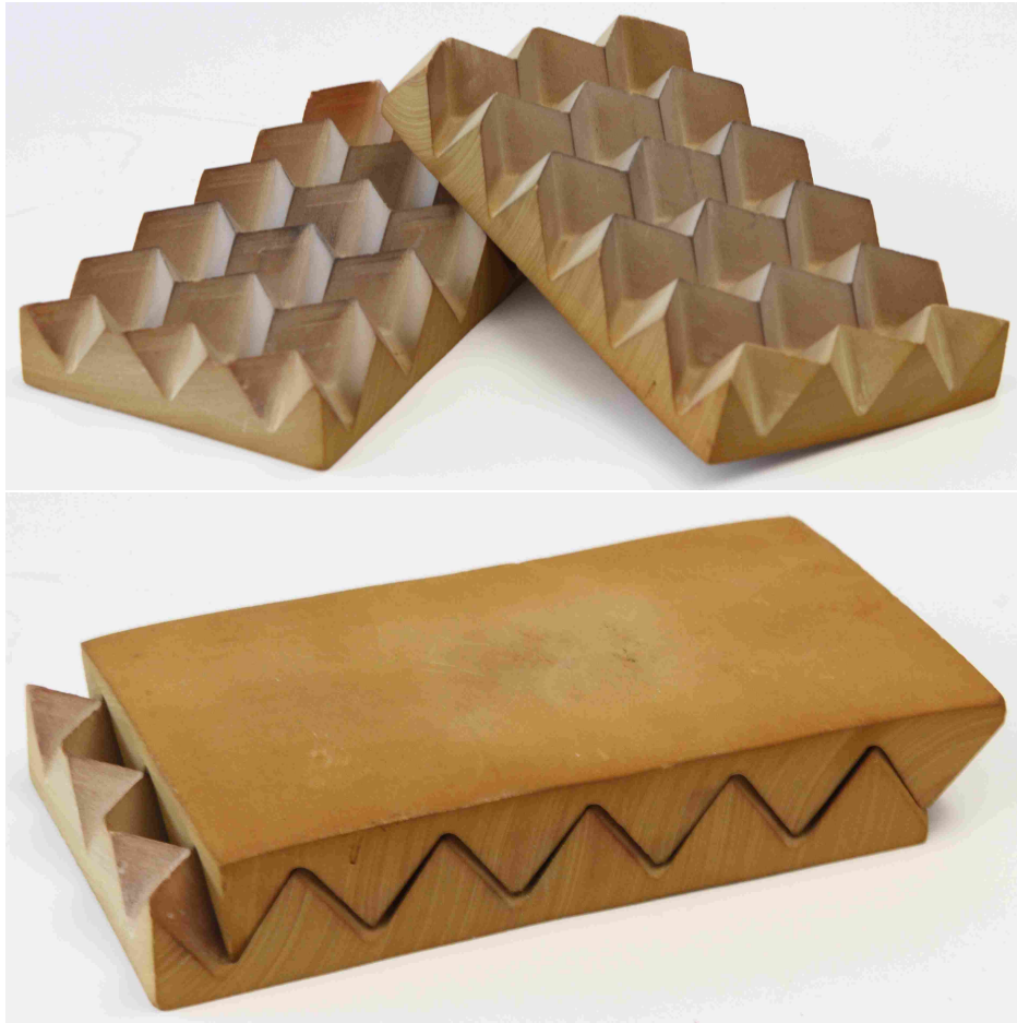
Figure 5.2: Two identical mold halves used for creating a Miura-ori pattern using the double mold process shown open and together.
