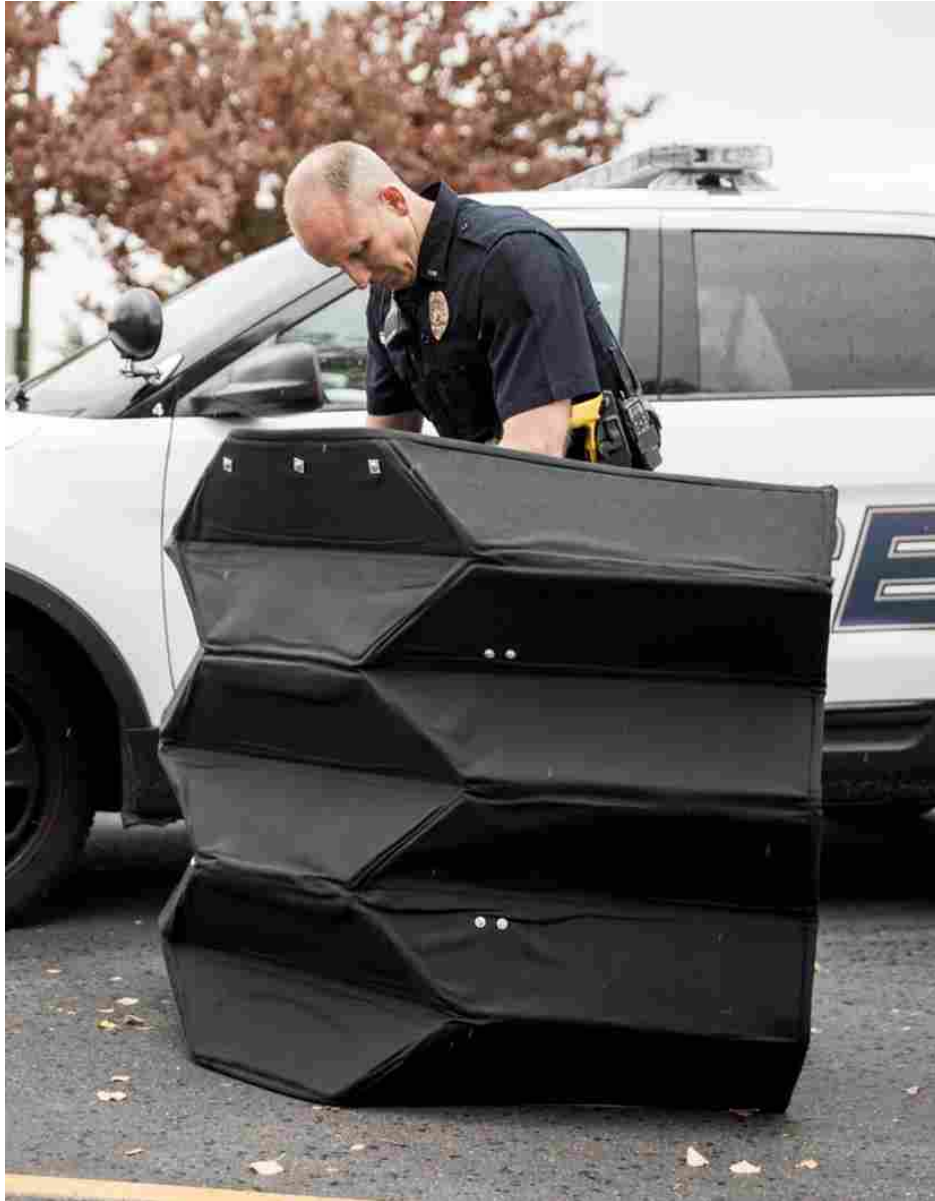
Figure 5.5: Origami-inspired ballistic barrier in the deployed state.
