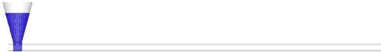
Figure 4-2: Geometry of the angled hopper with the same amount of mass and same boundary and initial conditions as the original gravity-fed system discussed in Section 4.1.
