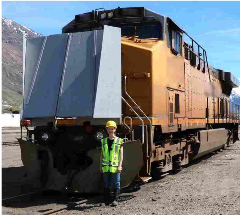
Figure 6.18: The top of the fairing stands 3.6 meters tall from the ground. An 158 cm tall person provides a visual indication of the fairing size. Photo has been modified to remove locomotive identity.
