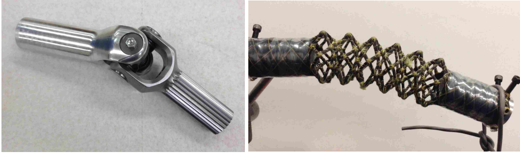
(a) Aluminum and steel universal joint. (b) Prototype 6 node, 2.5 inch compliant joint.
