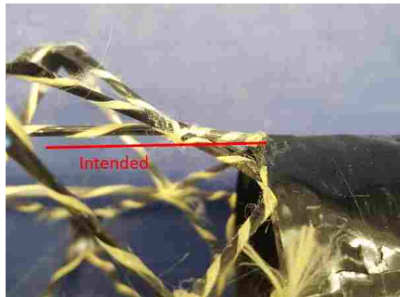
Figure 3.7: Detailed view of the longitudinal member as manufactured compared to the intended path.
