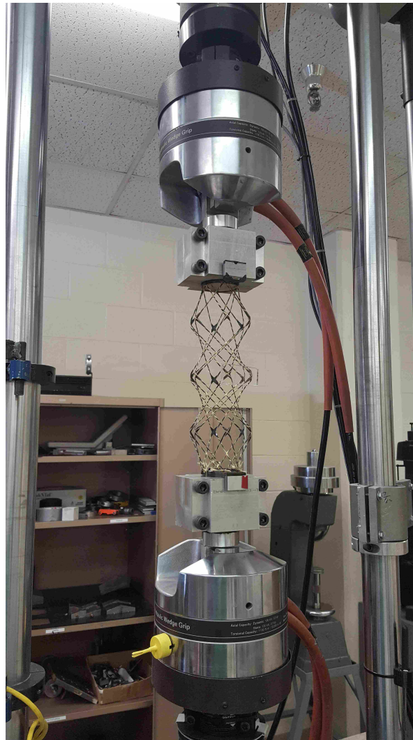
Figure 3.13: Torsion test fixture.
