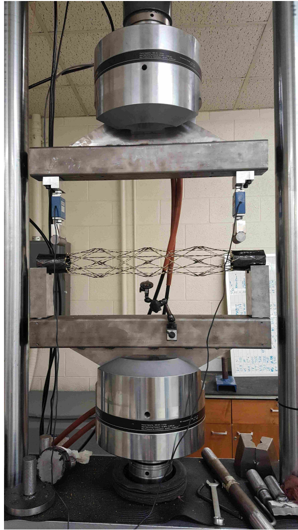
Figure 3.11: The intended four point bend fixture.
