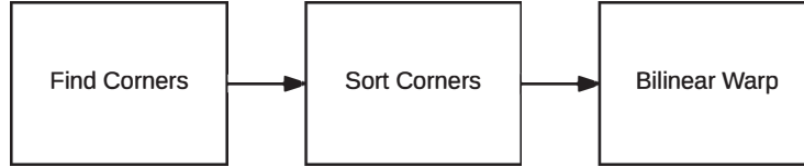
Figure 3.7: High-level preprocessing algorithm for bilinear image warping. The purpose of preprocessing each image is to scale each image into a standard shape and to remove as much white space as possible so only the blade is used for feature extraction.
