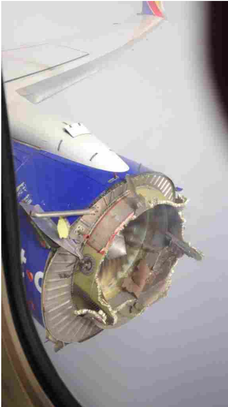
Figure 1.1: Catastrophic engine failure during Southwest flight 3472. Courtesy USA Today [1].
