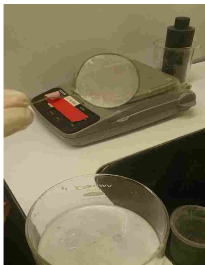
Figure A-5: The emulsion can be applied to the sample via a wire loop. This picture was taken after the process was completed; the lights should not be on. The white emulsion is starting to turn dark after just a few seconds of light exposure.
