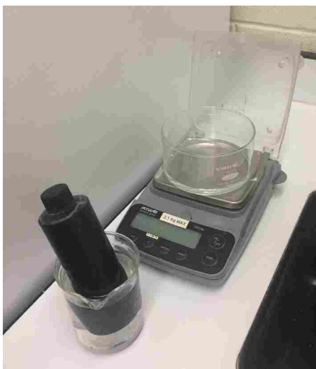
Figure A-4: The black bottle of AgBr photographic emulsion is resting in hot water. 10 g of the liquefied emulsion will be mixed into the container resting on the scale to make the final film solution.
