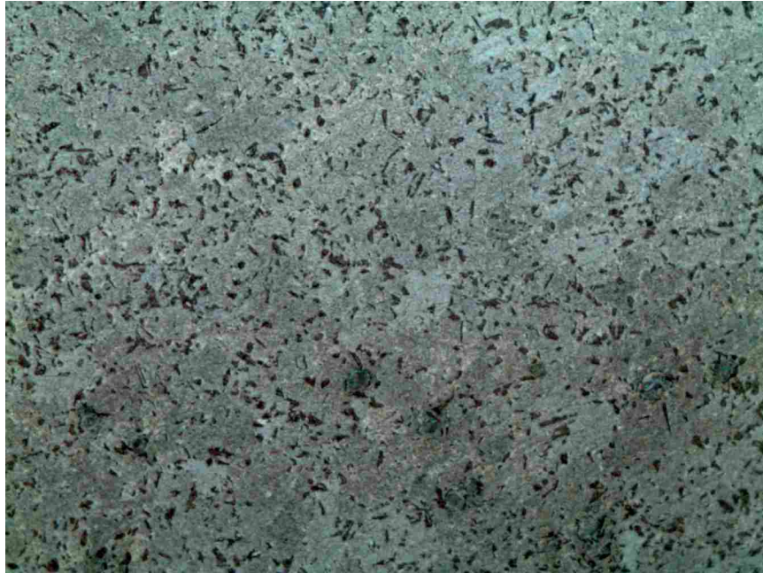
Figure A-6: This is a microprinted sample of TRIP steel under a light microscope at approximately 2,500 X magnification. Microstructural features are just visible, as there are some regions not covered with silver particles.
