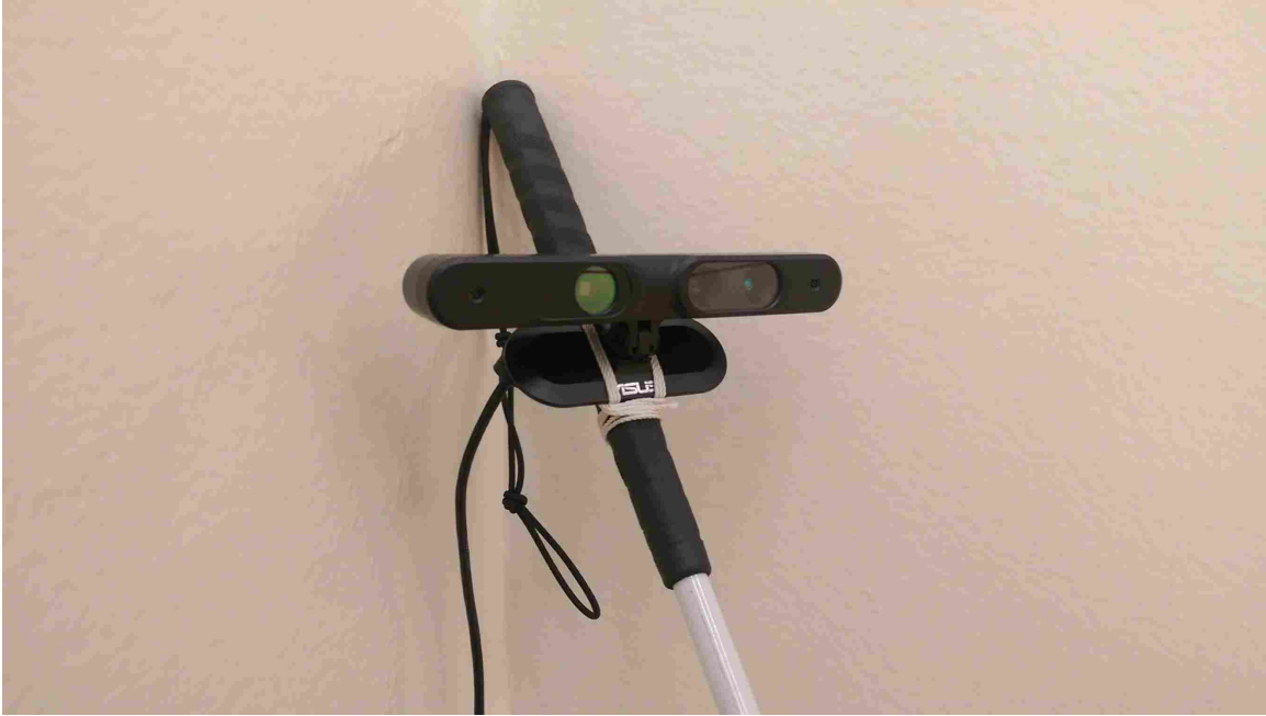
Figure 2.2: The Asus Xtion Pro Live is attached to the long white cane handle.
