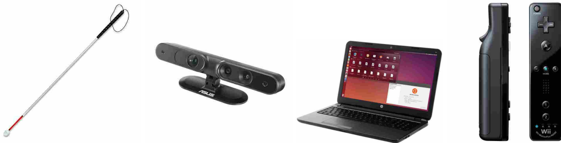
Figure 2.1: Pictured from left to right are the long white cane, Asus Xtion Pro Live, HP EliteBook 850 running Ubuntu 16.04, and Nintendo Wii remotes. The cane directs the sensor's field of view. The HP laptop processes the point cloud and informs the user of obstacles through the Wii remote rumble feature.
