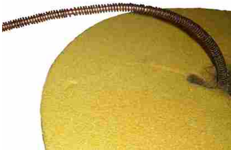
Figure 2.6: A photo of the nichrome wire wrapped around copper tubing. Note that for many of the experiments only nichrome wire was used to heat the transfer lines with no copper in between.
