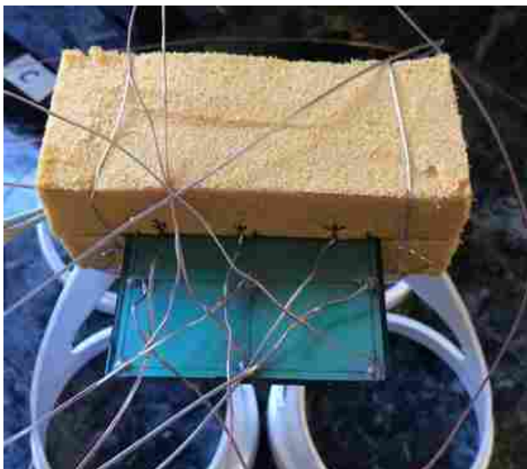
Figure 2.11: Replica experimental system partially insulated with thermocouples attached to the silicon surface.
