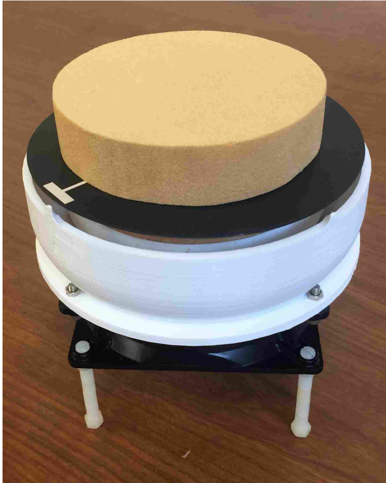
Figure 2.10: Assembled spiral system atop the fan duct and cooling fan.
