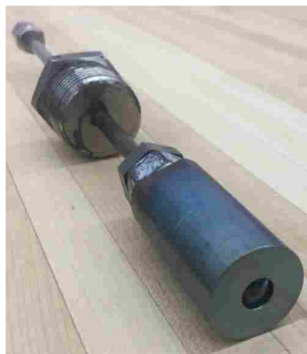
Figure 19: Isometric view of the optical probe without the 1.59 mm diameter flexible tubing or sapphire fiber (8 and 10 from Figure 17).
