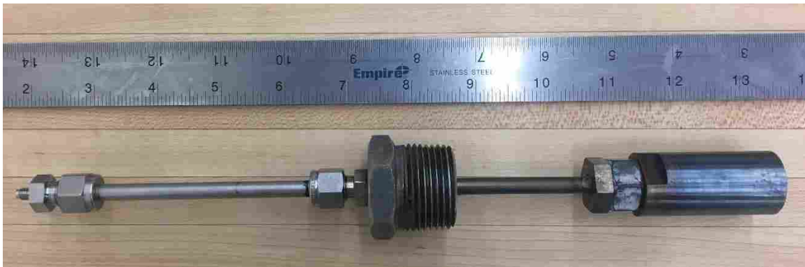
Figure 18: Top view of the optical probe without the 1.59 mm diameter flexible tubing or sapphire fiber (8 and 10 from Figure 17).
