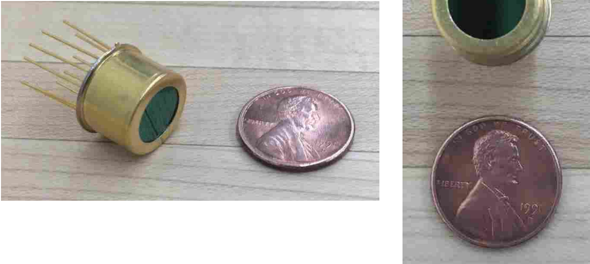
Figure 15: Quad (four element) InGaAs detector containing filters representing ISBR bands C, E, B1, and B2. A penny is included for a reference of scale.
