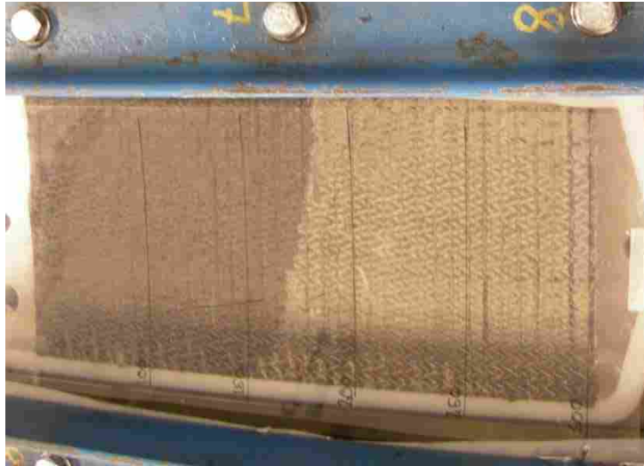
Figure 2-1: Top view of a 1D flow test for fiber glass. Flow is shown from left to right
