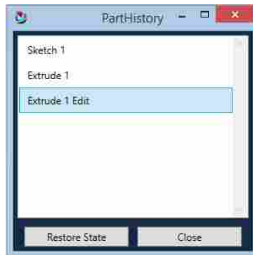
Figure 4.3: Image showing the GUI and some revisions for a part with a button to restore the part to different revisions and close the window.
