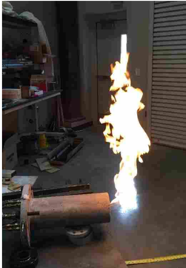
Figure 4-6: Preliminary Burner Testing at 50 KW_{th} .
