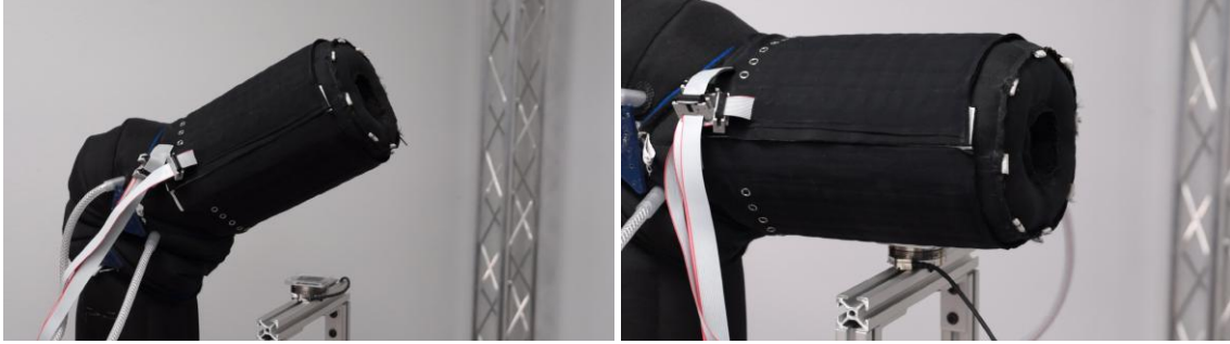
Figure 2.11: Images of tactile sleeve integrated onto a single link robot arm and the tactile sleeve being pressed against the force-torque sensor.
