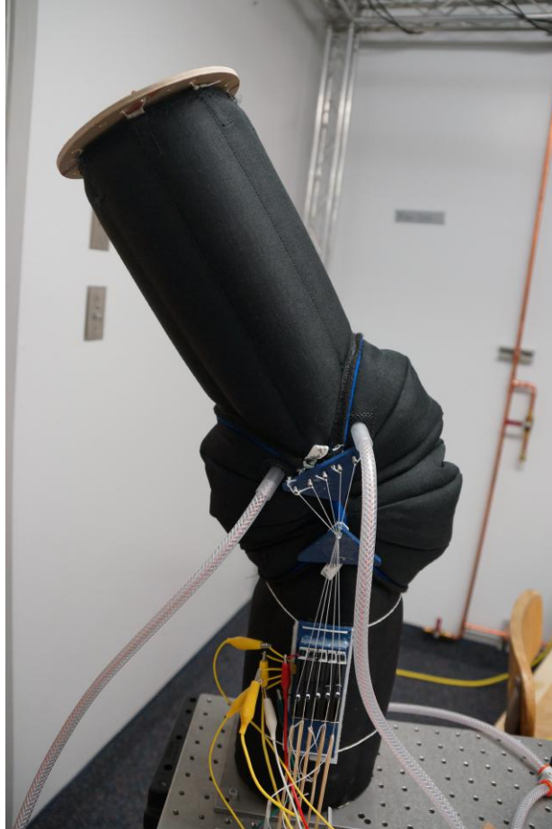
Figure 3.1: The Grub: a single link pneumatically actuated inflatable soft-robot.
