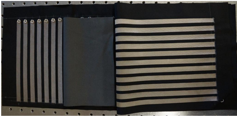
Figure 2.3: Sensor construction with columns and rows of conductive fabric. The gray resistive material is folded back to reveal columns of conductive material. Metal snaps are located at the top of each column.
