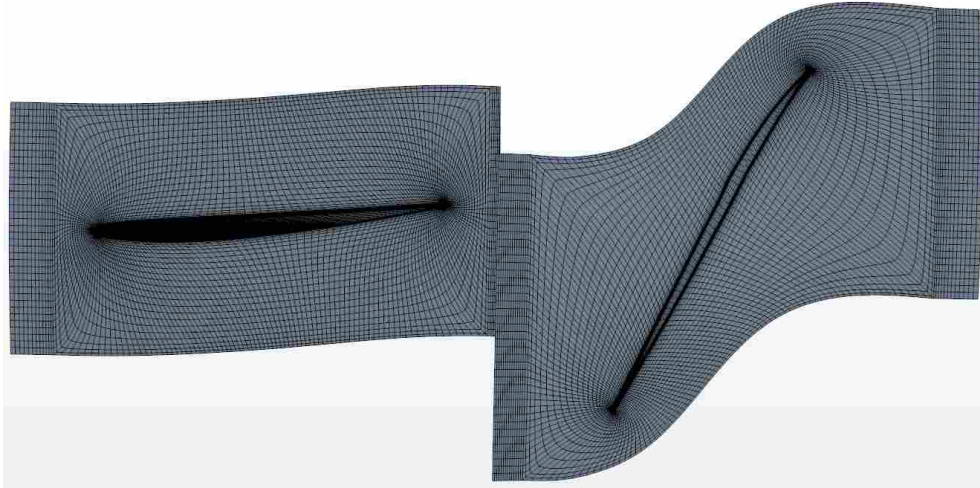
Figure 3.16: Top view of mesh for IGV (left) and NASA rotor 37 (right).
