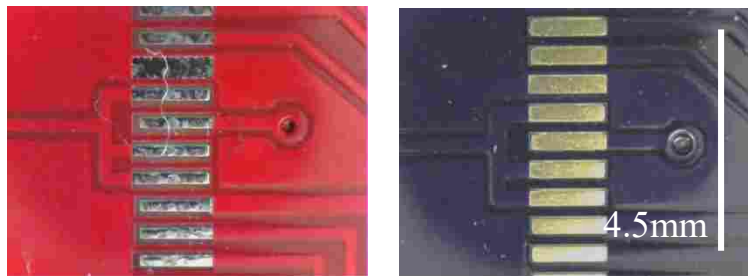
Figure 3-5: Image of original Diyouware PCB (left) and customized PCB (right). The pads on the updated version are bigger and more consistent.
