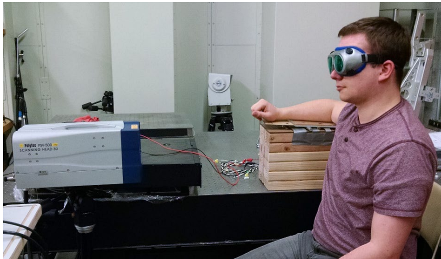
Figure 2-2: Polytec PSV-500-3D Scanning Laser Doppler Vibrometer
