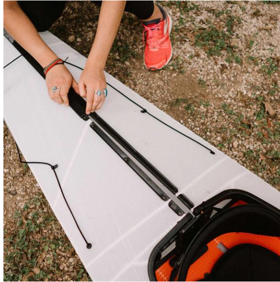
Figure 3.2: The origami kayak (Oru Kayaks™) uses several stability techniques such as supporting bulkheads, straps, and retaining channels to keep its folded state. Image downloaded from www.orukayak.com December 3, 2018.
