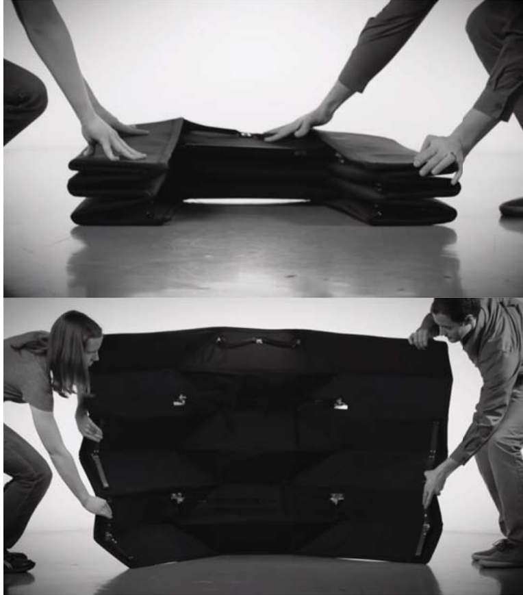
Figure 2.1: An origami-based ballistic shield in its closed state (top) and deployed state (bottom).
