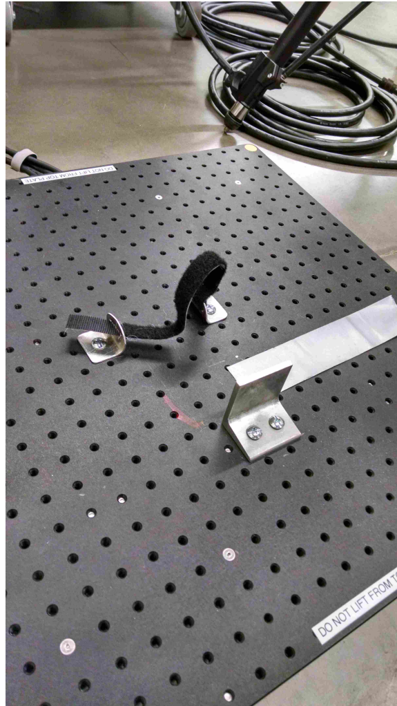
Figure 3.2: Modifications made to vibration platform to control location and movement of foot during testing
