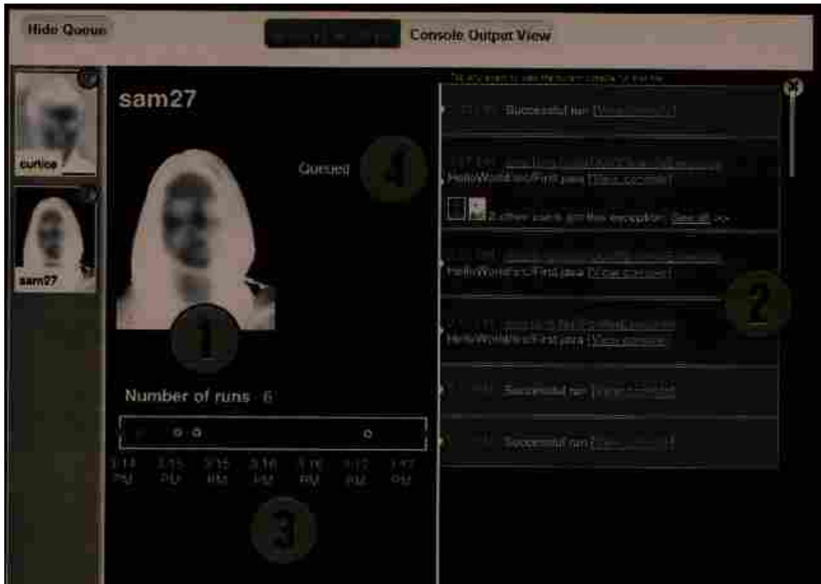
Figure 2.6: Student panel view from [4]. 1) shows the student’s image and name. 2) shows the event stream, including time stamps, errors, and exceptions. 3) shows a timeline indicating when successful and unsuccessful runs occurred. 4) indicates whether or not the student is on the help queue.
