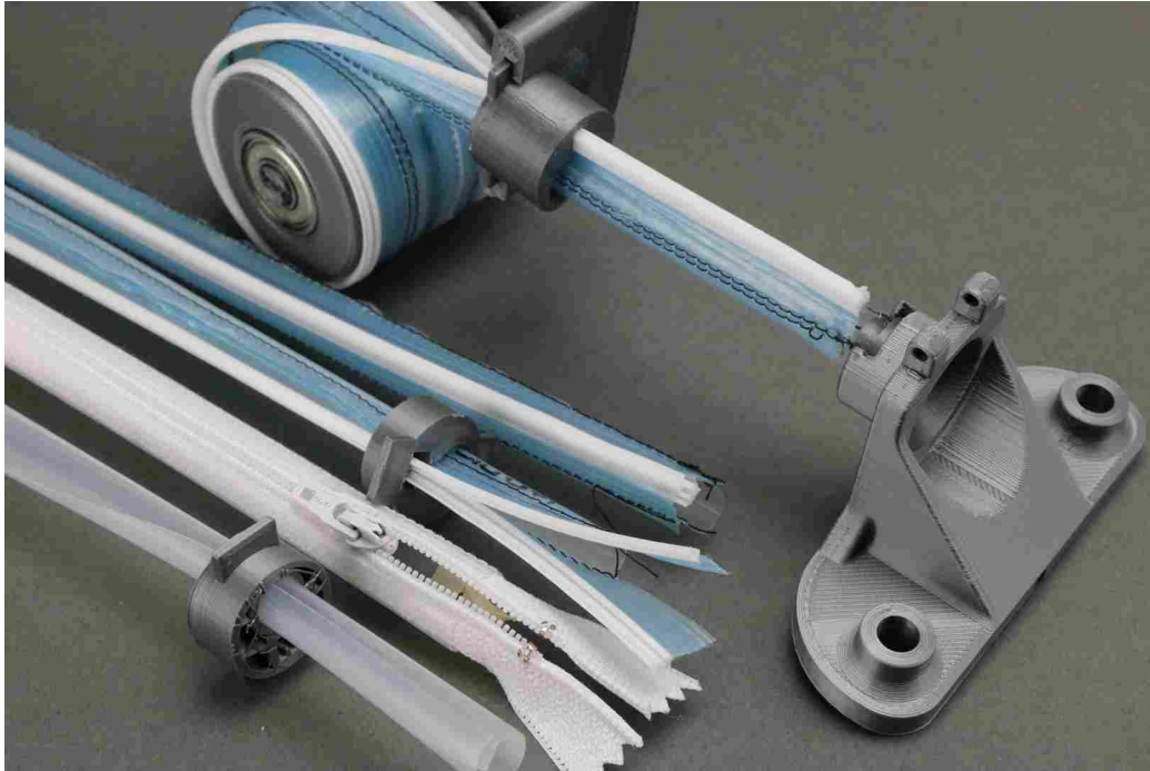
Figure 5.2: Tube concept progression with early prototypes on the left progressing to the final testing prototype on the right.
