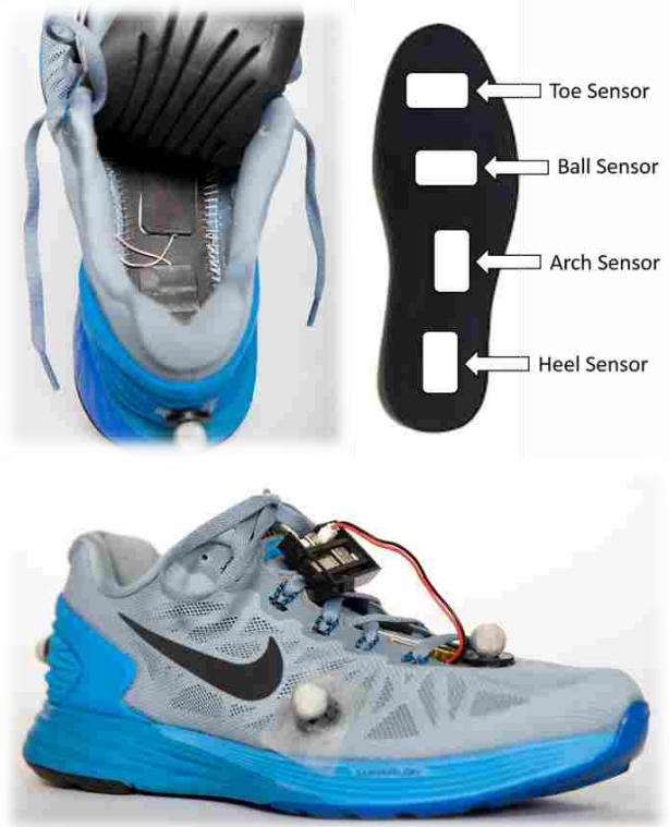
Figure 3-2: The shoe that was instrumented with the nanocomposite piezo-responsive foam sensors, microcontroller, and battery. The sensors were embedded under the insole at the heel, arch, ball, and toe positions and the reflective markers were placed at the heel, toe, and lateral positions for motion capture.
