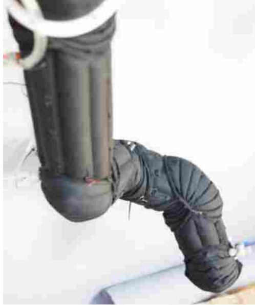
Figure 1.1: This fully inflatable manipulator developed by Pneubotics was designed using optimization techniques presented in this work.
