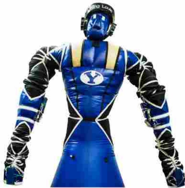
Figure 1.3: A pneumatically actuated robot with fabric-based limb and body structure.
