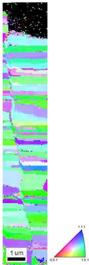
Figure 4-11: IPF map of a portion of FIB-prepared wedge taken from an unannealed wire showing the small grain size.
