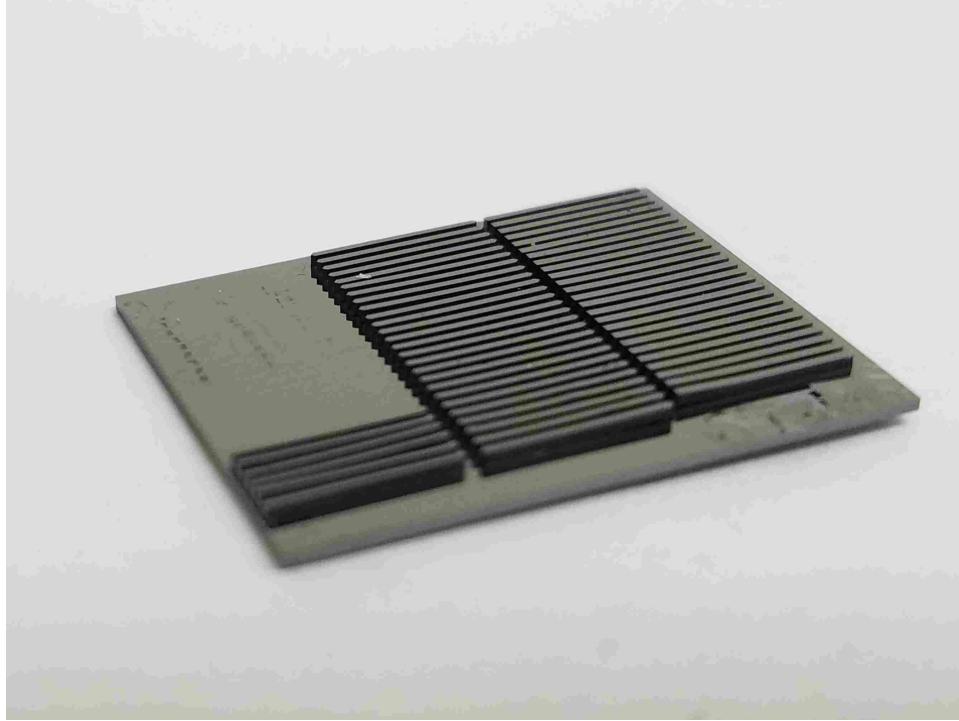
Figure 2.2: Grown and infiltrated carbon-nanotube beam structures with some beams already removed.
