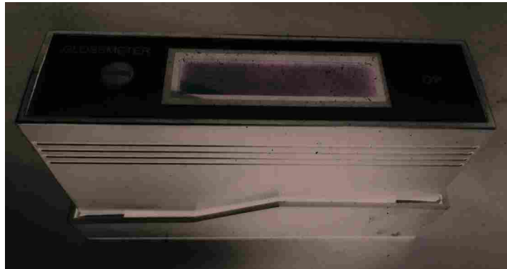
Figure 4.1: Image showing the gloss-meter. The gloss-meter was used to independently measure the measured gloss and haze of samples.
