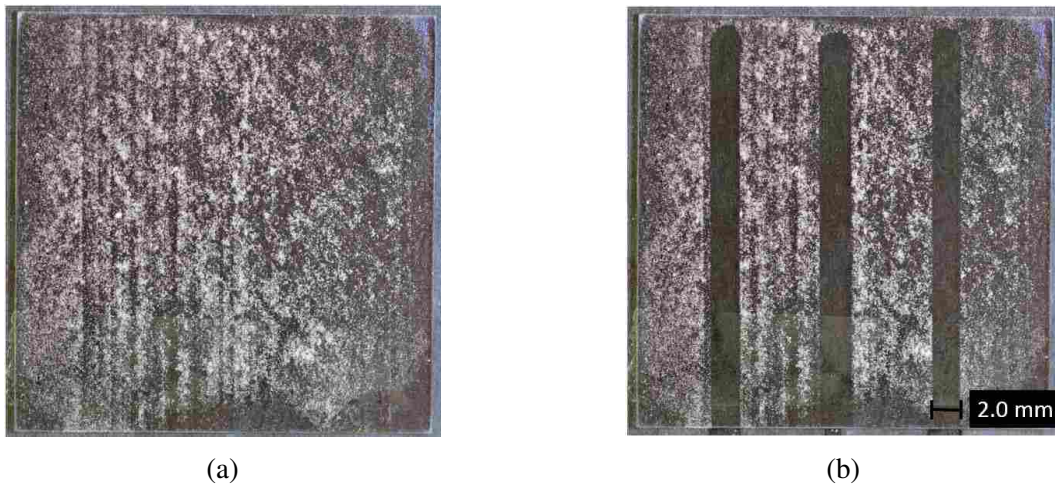
Figure 2.4: One a distinct feature of self-cleaning is the droplet path, which is where particulates have been removed from the surface after water droplets roll over the surface. (a) Shows a surface with salt particles loosely placed on the surface. (b) Shows the same surface as (a) after 2 mm water droplets rolled over the surface.
