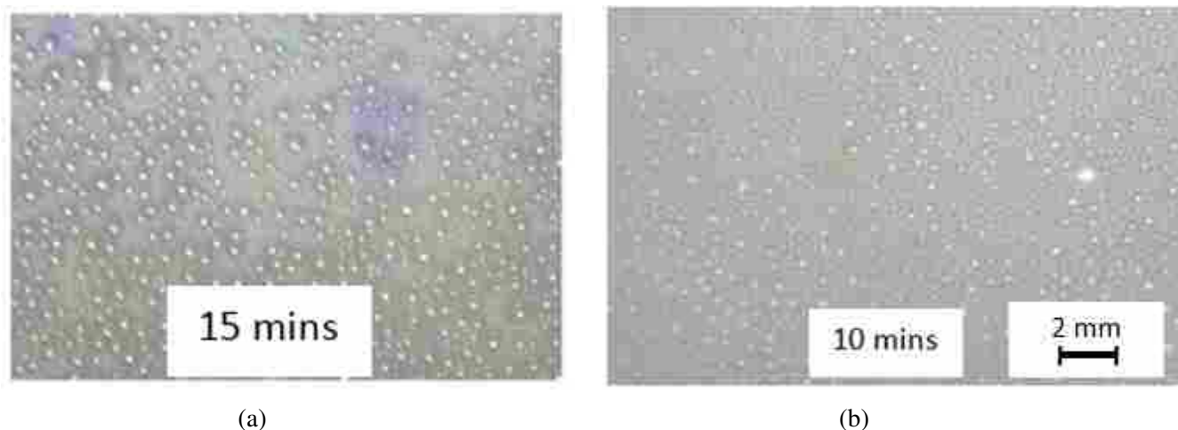
Figure 3.12: Condensation on two nano-structured surfaces contaminated with salt particles (a) and tobacco residue (b). As can be seen in this image, the particles on the surface initially serve as the primary nucleation sites for condensing droplets.
