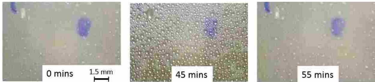
Figure 3.10: Sequence of images showing an abbreviated condensation cycle occurring on a surface contaminated with salt, where the droplets do not reach the critical diameter to roll off the surface. Because the droplets do not roll off the surface, the surface does not exhibit self-cleaning properties. Note: time=55 mins is the same image as time = 0 mins in Figure 3.9.
