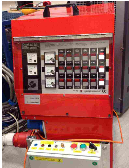
Figure 6.2: The high power load bank used for initial controller testing with the converter.
