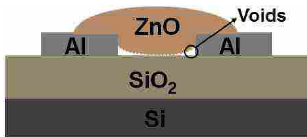
Figure. 8.8. Possible ZnO TFT architecture following deposition of ZnO by drop-casting.
