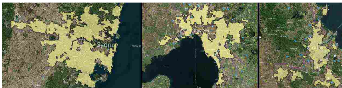
Figure 4.5: Estimates of Optus' HFC network coverage in Sydney, Melbourne and Brisbane
