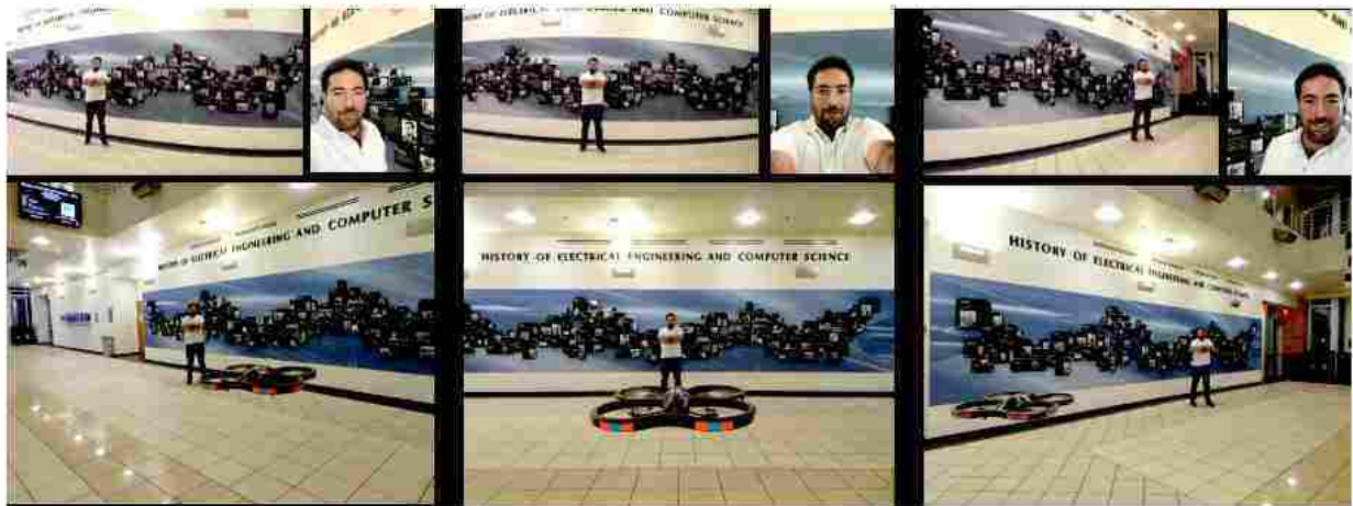
Figure 6.10: Testing with Parrot ARDrone 2.0 in indoor real-world environment though assigning three different vantage points using a SMD and transforming them to correspondents from the drone perspectives for taking the long-range selfie.
