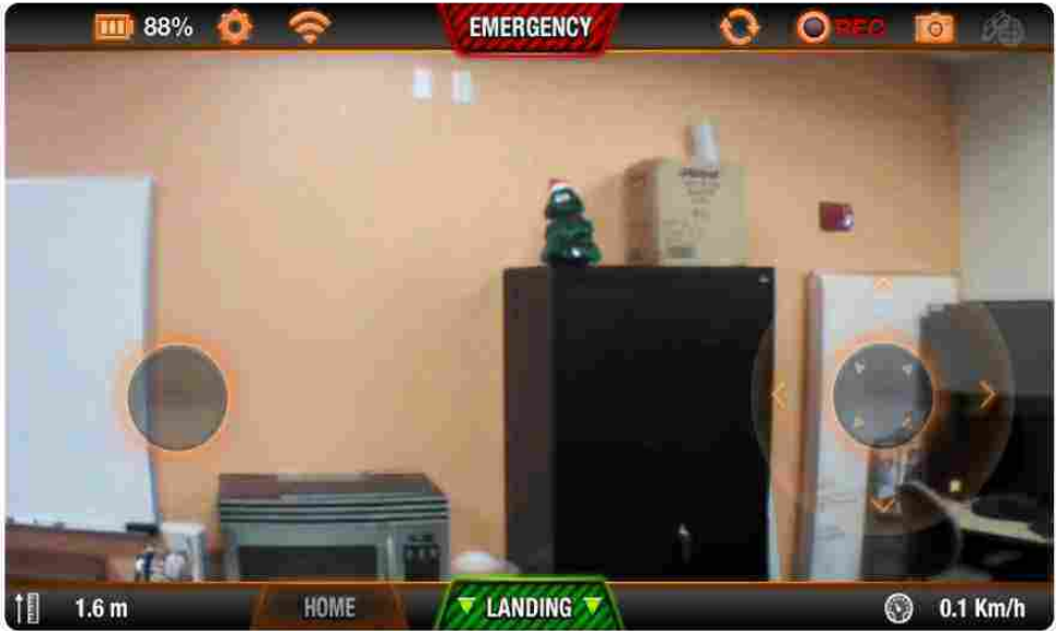
Figure 4.8: Piloting the quadcopter using AR.FreeFlight user interface. Mobile device IMU and touch-based gestures are used to control the quadcopter.
