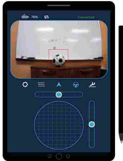
Figure 4.1: The upper part of the interface broadcasts the image stream from the quadcopter frontal camera. The user can select a target by drawing a bounding box over the camera view. After selecting the required object and starting the semi-autonomous mode, the upper part switch to stream the processing frames and shows the auto-selected part to the user. Switching between the manual pilot and the human-guided pilot can be done at any time to and the object selection as well. The human can directly control the quadcopter by sketching on the lower control panel.
