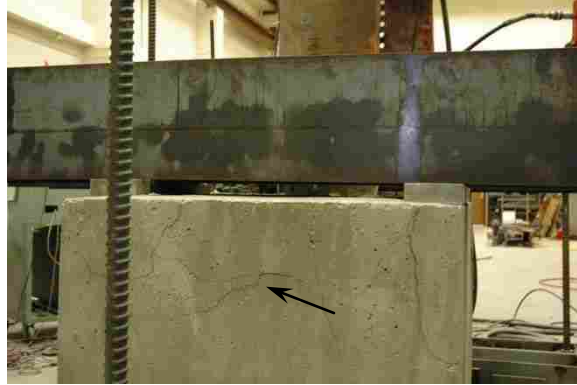
Figure 4-8: Cracking at the End of Specimen 2 After Testing (North-South)
