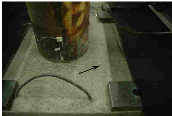
Figure 4-6: Initial Cracking of Specimen 2 (East-West)
