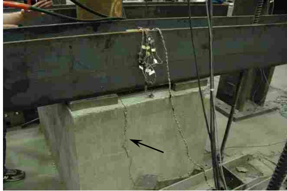
Figure 4-4: End of Cap of Specimen 1 After Testing (North-South)
