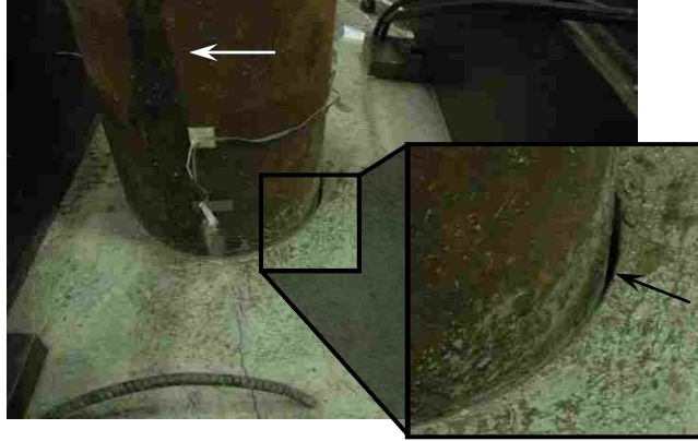
Figure 4-1: Gap in Specimen 1 [249 kN (56 kips), 5.3 cm (2.1 in)]
