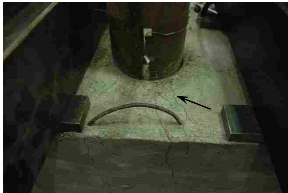
Figure 4-3: Specimen 1 at Maximum Displacement (East-West)
