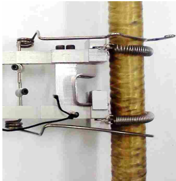
Figure E.6: Extensometer Attached to Specimen with Wire Clips and Springs
