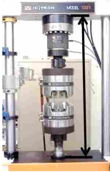
Figure E.8: Total Machine Displacement (See Arrow)
