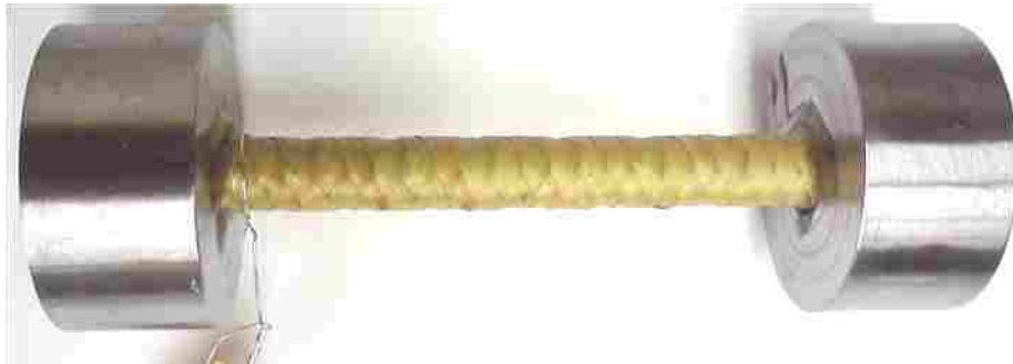
Figure 3.14: Typical Specimen Set in End Caps
