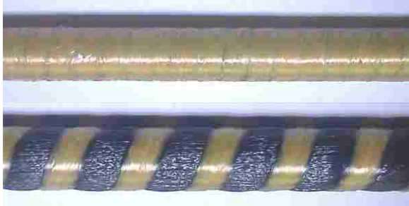
Figure 2.5: Spiral Sleeve: A) Full Coverage (Top); and, B) Half Coverage (Bottom)
