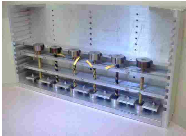
Figure 3.15: End Cap Setting Fixture: A) Computer Rendering (Top); and, B) Manufactured Fixture (Bottom)
