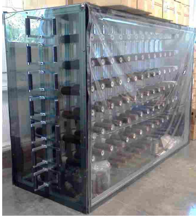
Figure 3.4: Fiber Creel Loaded with Basalt and Protected by Plastic Covering
