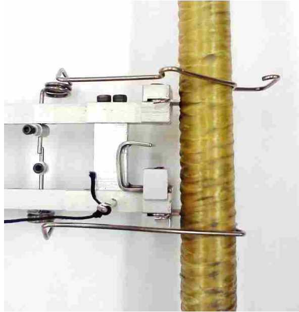
Figure E.5: Extensometer Attached to Specimen with Wire Clips
