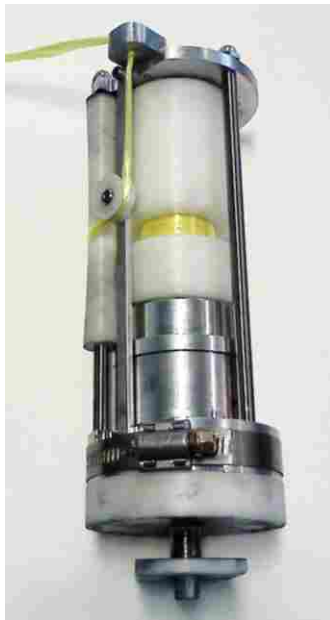
Figure 3.2: IsoTruss Bobbin Loaded with Aramid Spool
