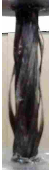
Figure E.2: Typical Specimen with a Ballooned Sleeve
