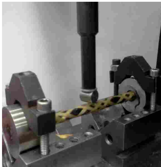
Figure 3.27: Photo of Specimen at Impact
