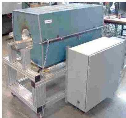
Figure 3.8: SPX Lindberg Model 54977 Curing Oven
