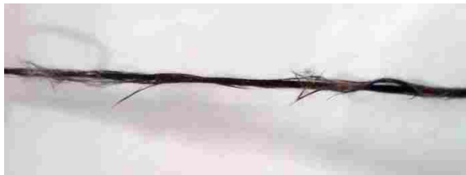
Figure 2.1: Damage to Fibers Used for the Sleeve
