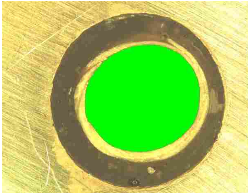
Figure 3.17: Typical Specimen Cross-Sectional Area Measurement
