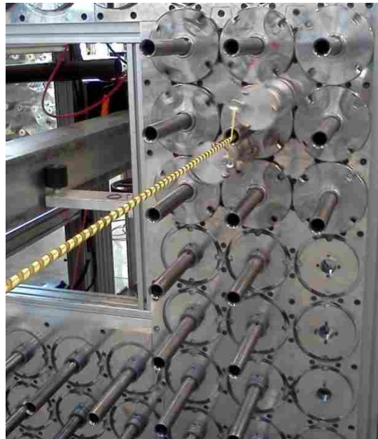
Figure 3.7: Core Material Being Consolidated by the Sleeve
