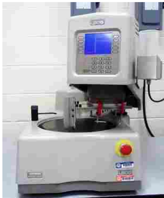
Figure 3.13: Specimen End Sanding Fixture Attached to the Spectrum System 2000 Sander
