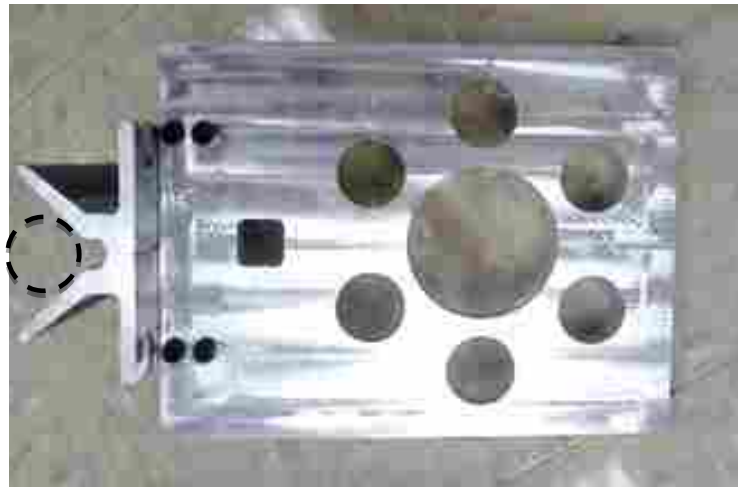
Figure 3.12: Specimen End Sanding Fixture
