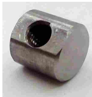
Figure 3.25: Cylindrical Tup Used to Impact Specimens
