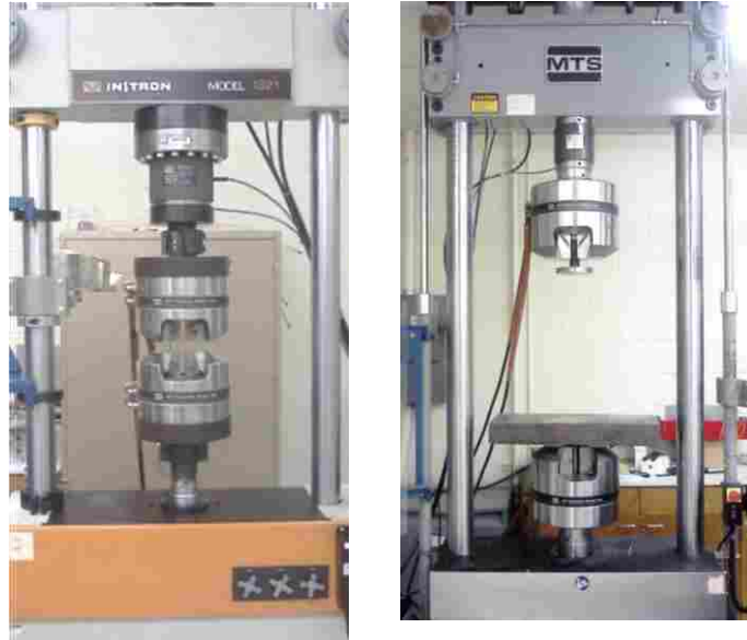
Figure 3.29: Compression Machines: A) 90 kN (20 kip) Instron (left); and, B) 489 kN (110 kip) MTS
