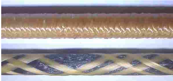
Figure 2.7: Braided Sleeve: A) Full Coverage (Top); and, B) Half Coverage (Bottom)
