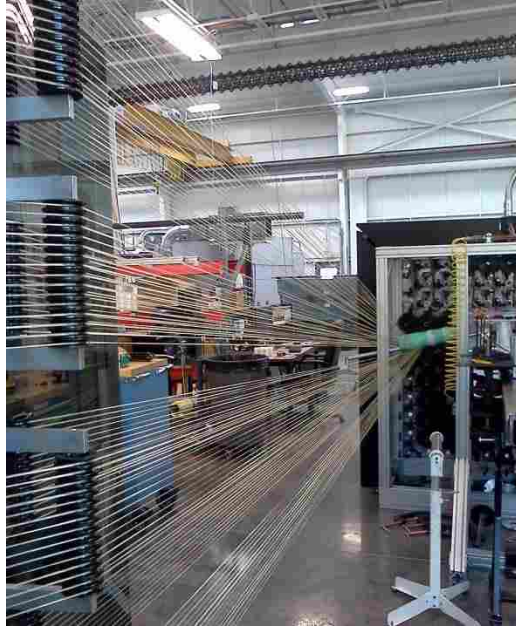
Figure 3.6: Core Material Traveling from Fiber Creel to the Machine Wall
