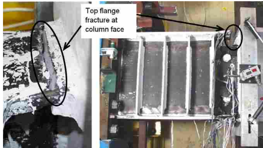
Fig. 1-5 Fracture of specimen MWS at the link-to-column connection [13]
