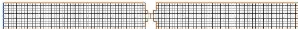
Figure B-4: Plan View of the Flume with a Short Abrupt Contraction
