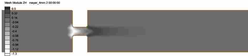
Figure C-57: Plan View of the Final Bed Elevations for a 48 Hour Simulation of the Wide Flume with an Abrupt Contraction Test Case using the Meyer-Peter & Muller Method with the 4.0mm Particle Size
