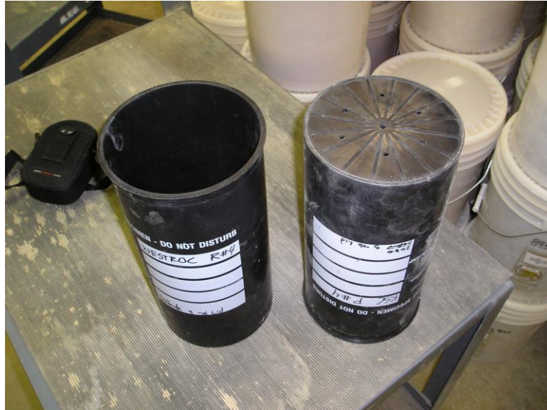
Figure 3-2: Pre-drilled plastic molds.
