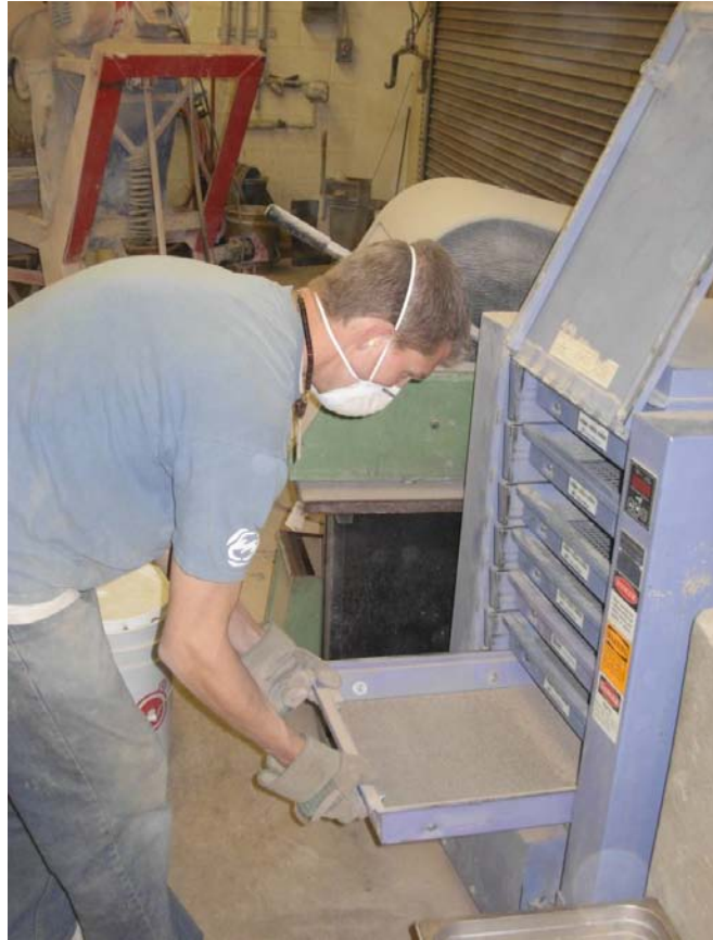
Figure 3.2 Operation of the sieving machine for bulk material separation.
