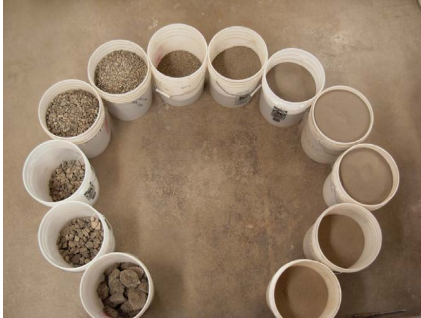
Figure 3.3 Road base separated after bulk sieving.
