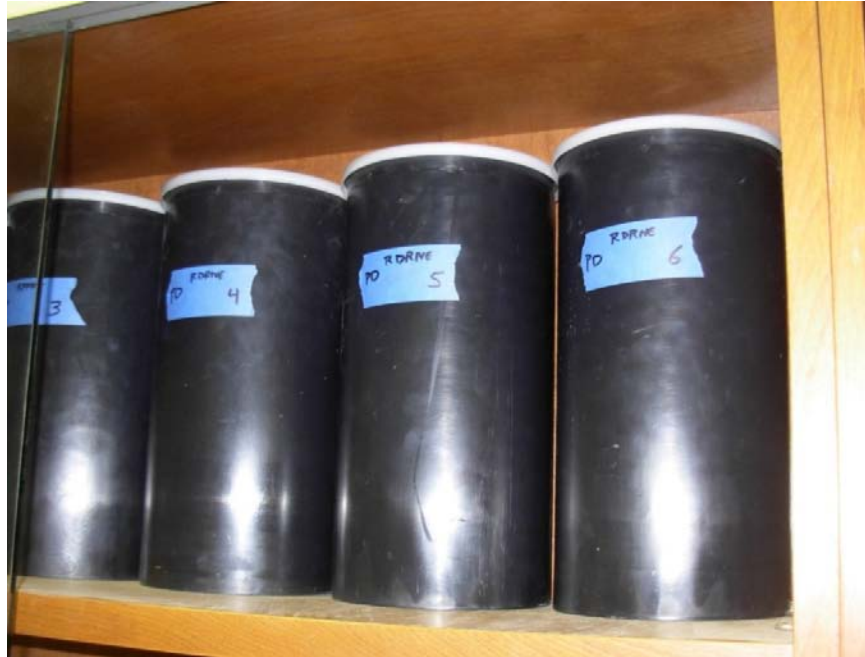
Figure 3.7 Road base moistening in sealed plastic cylinders.
