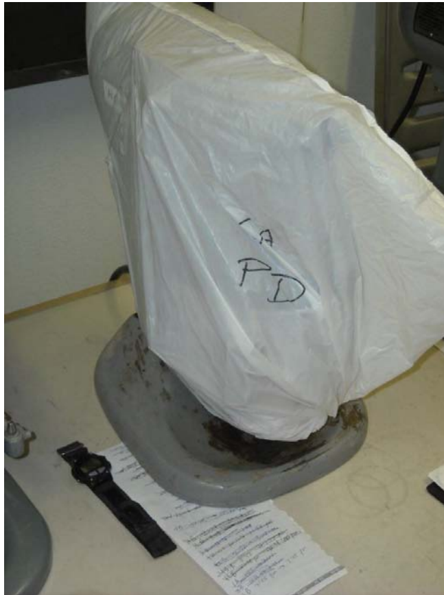
Figure 3.12 Slurry aging in a covered mixer in a temperature-controlled environmental chamber.
