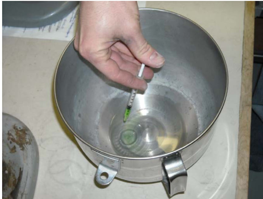
Figure 3.9 Addition of a set-retarding, water-reducing admixture to cement slurry water.
