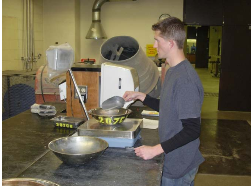
Figure 3.6 Proportioning of road base aggregate for testing.
