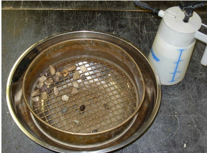
Figure 3.4 Aggregate during washed sieving for road base classification.
