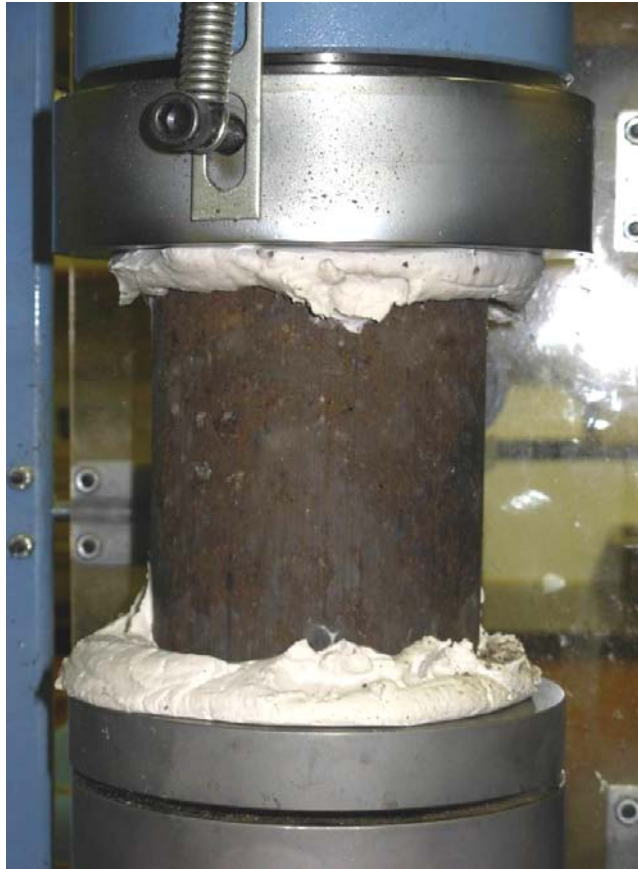
Figure 3.19 CTB specimen undergoing 7-day UCS testing.
