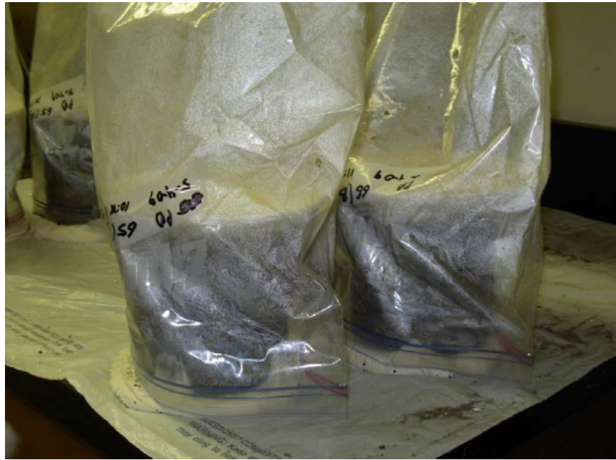
Figure 3.18 Hardening of gypsum caps in preparation for 7-day UCS testing.
