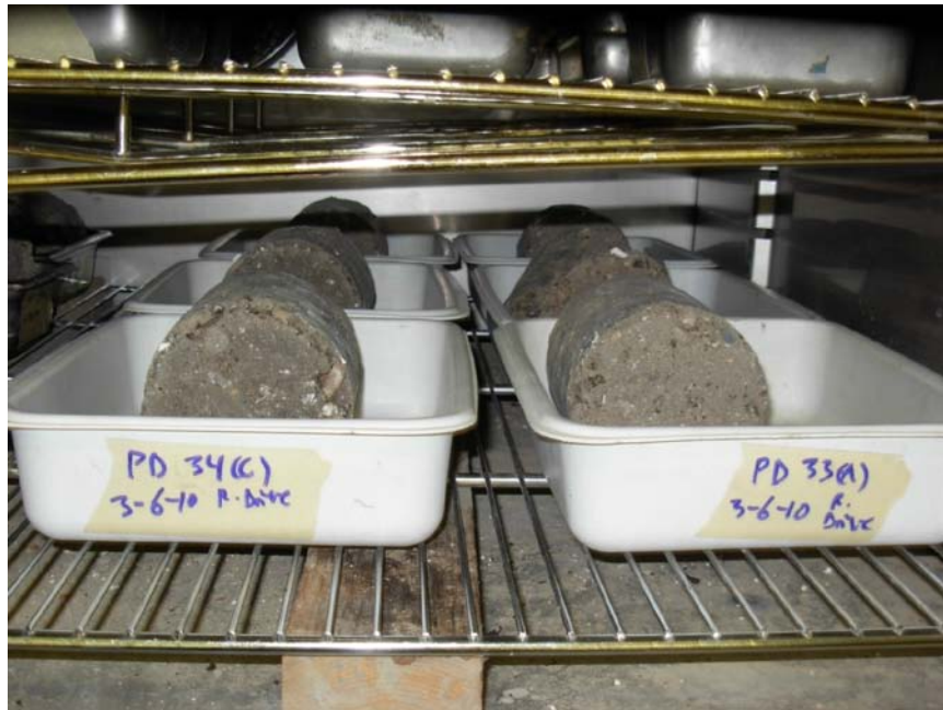
Figure 3.20 Specimens drying in a 140°F oven in order to obtain DD and MC.
