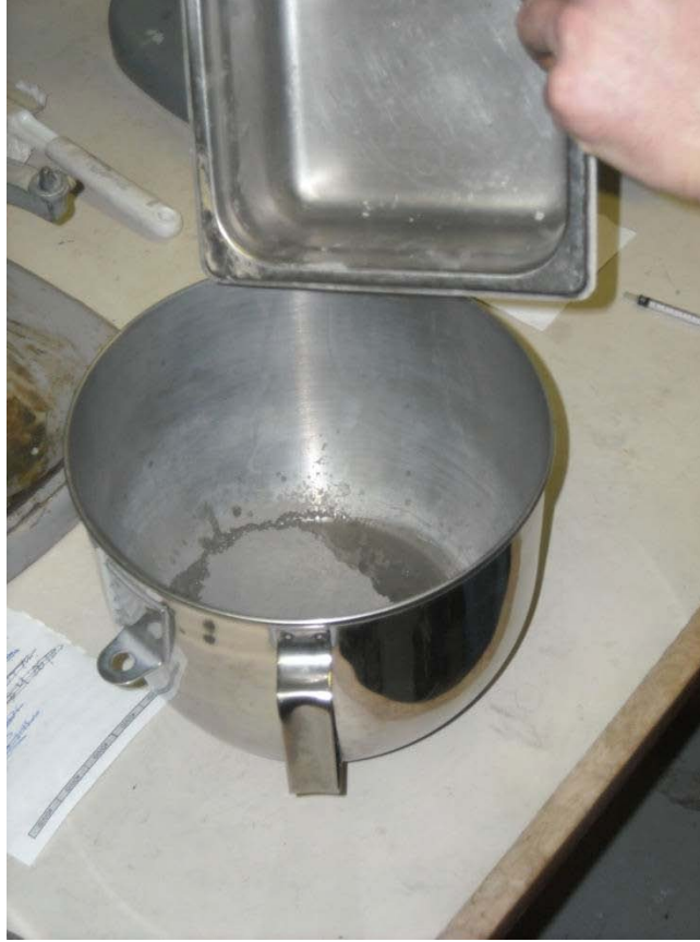
Figure 3.10 Addition of cement to water to prepare cement slurry.
