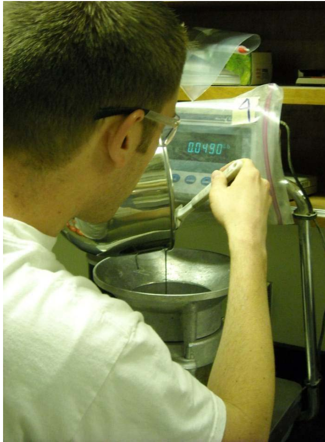
Figure 3.13 Adding cement slurry to aggregate.
