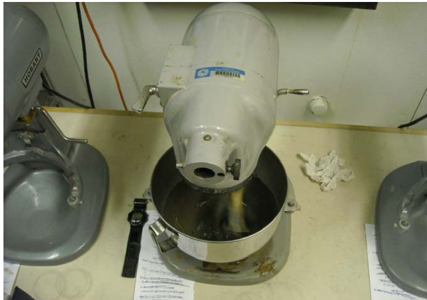
Figure 3.11 Initial mixing to prepare cement slurry.
