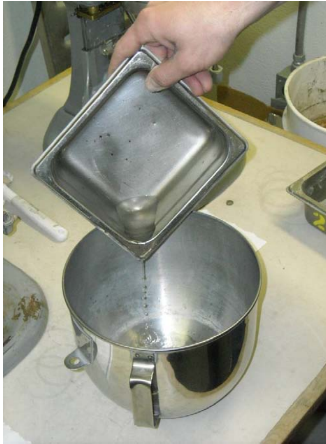
Figure 3.8 Conditioned, deionized water used to make cement slurry.
