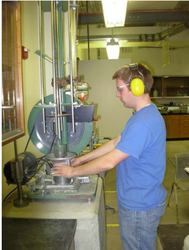
Figure 3.16 Compacting a CTB specimen.
