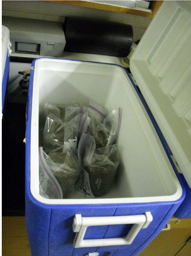
Figure 3.17 CTB specimens ready for 7 days of curing at room temperature.
