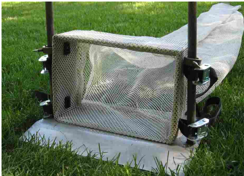
Figure 2-2. Bunte/Abt bed-load trap as it would be deployed on the streambed.
