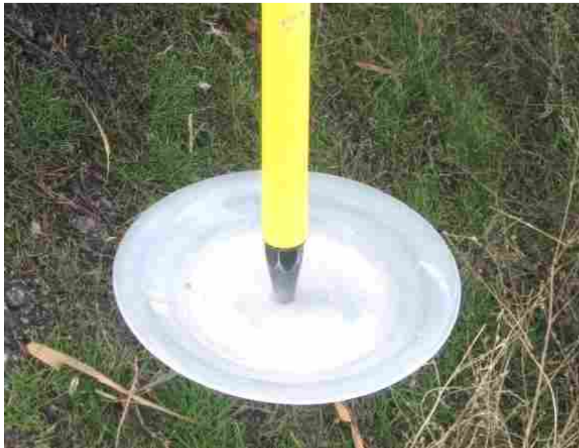
Figure 3-3. Dinner plate used to keep tip from sinking into the mud.
