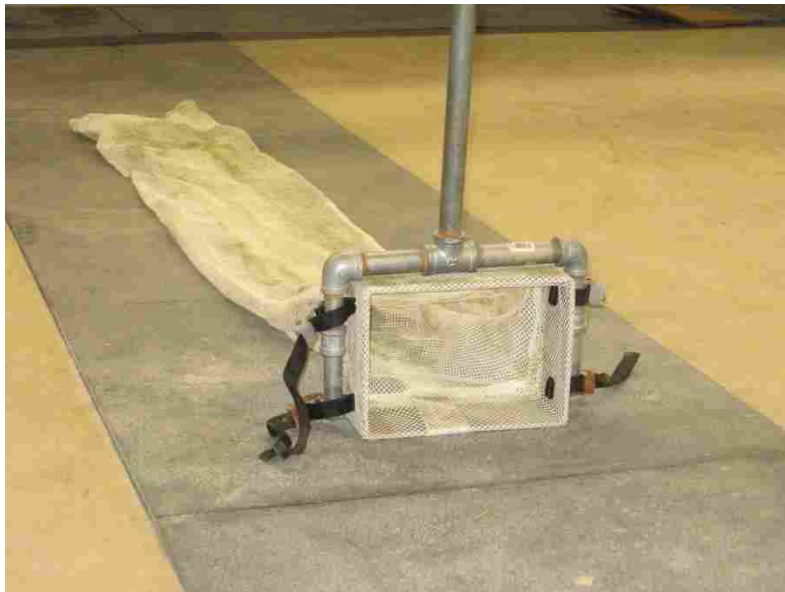
Figure 2-3. Handheld version of the Bunte-Abt trap nicknamed "Stanley Sampler".
