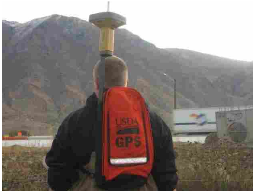
Figure 3-4. GPS mounted on backpack for automatic point reading.
