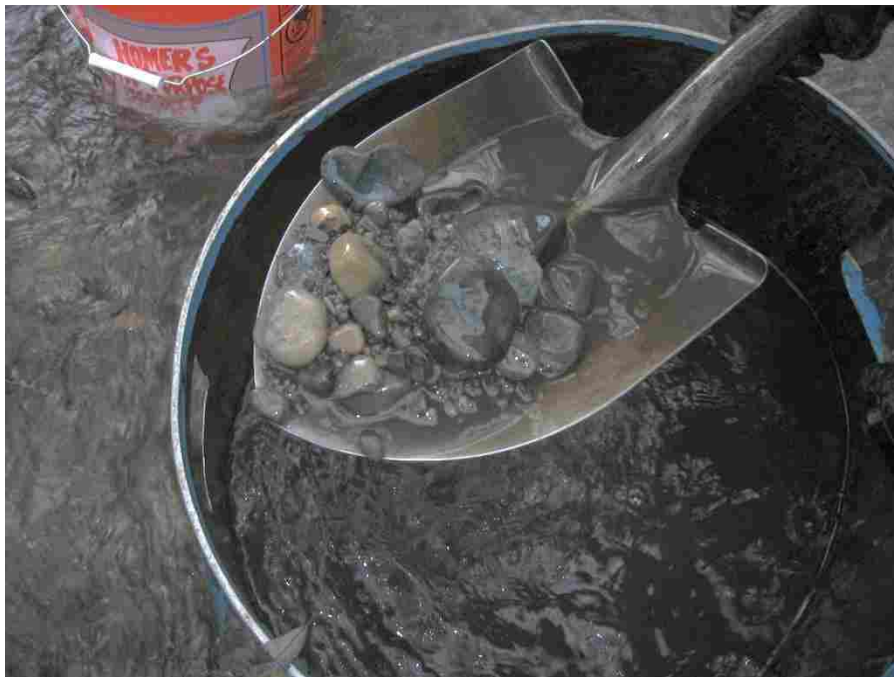
Figure 1-3. Subsurface sample taken from within a 55-gallon barrel flow shield.
