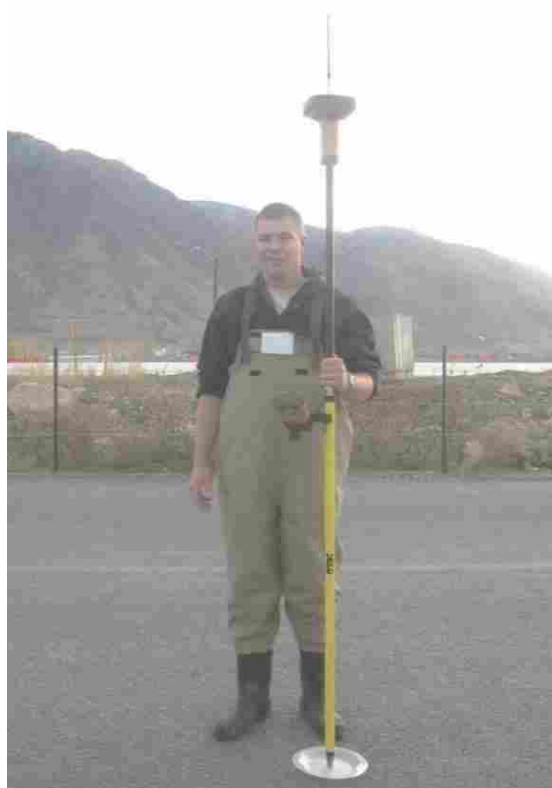
Figure 3-2. Survey rod with GPS unit and data collector.
